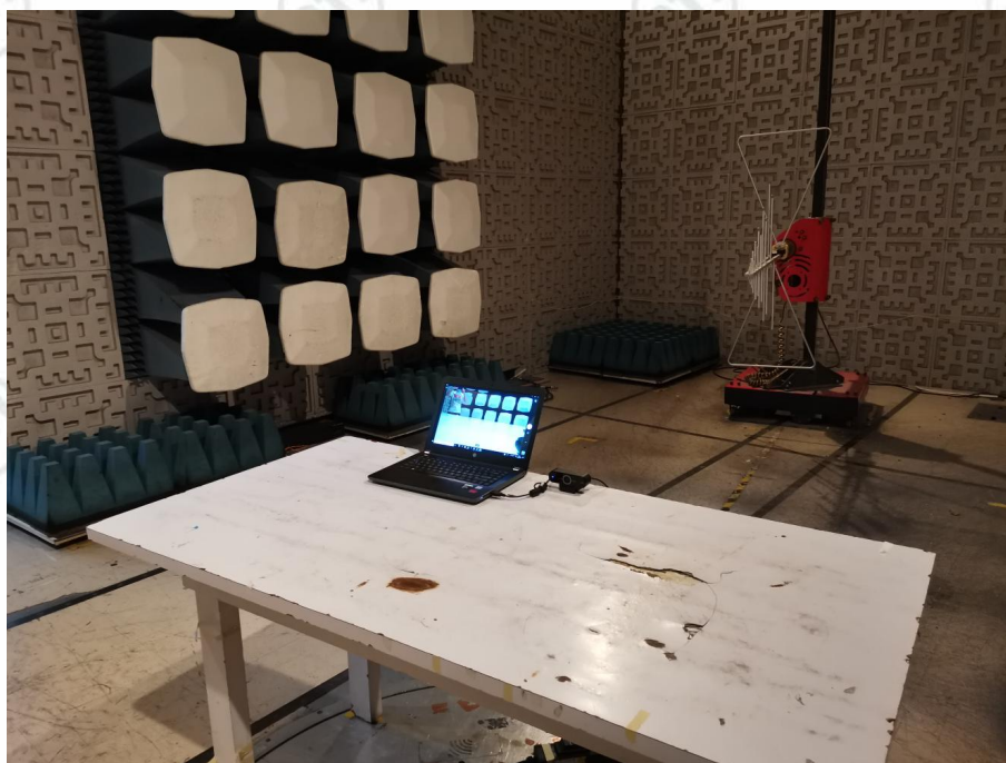
RADIATED DISTURBANCE TEST SETUP
