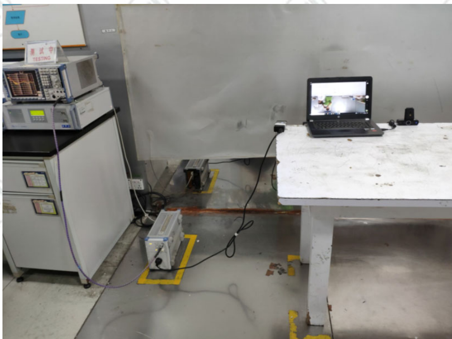
CONDUCTED DISTURBANCE TEST SETUP
