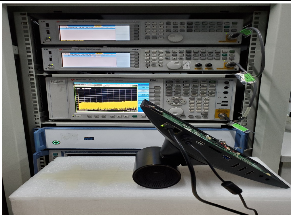
RF Conducted Test Setup
