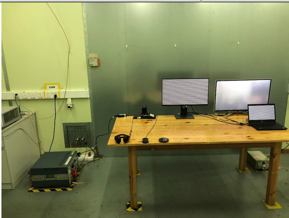
Conducted Emission Test Setup
