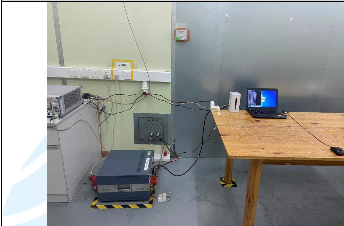
Conducted Emission Test Setup
