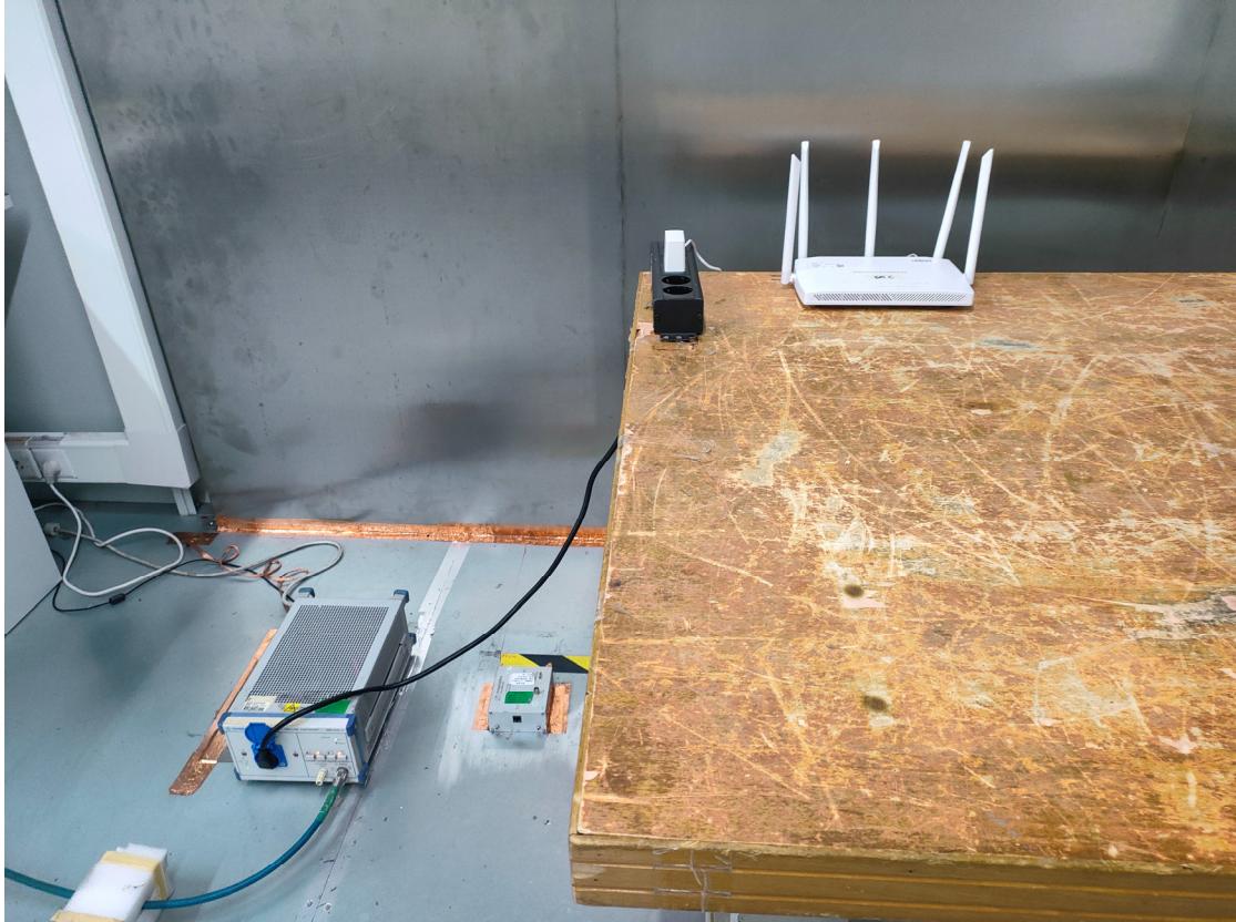
Conducted Emissions - Side View
