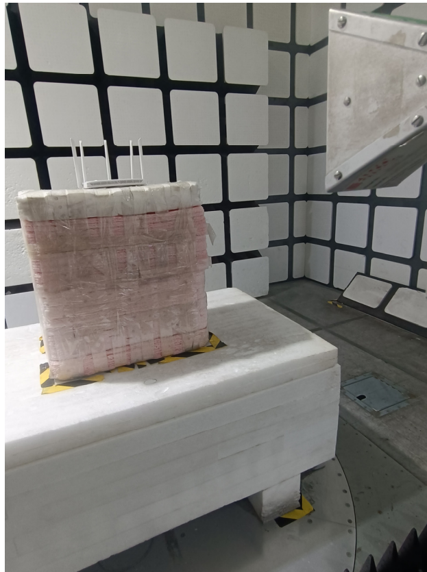
Radiated Emissions View (18-40 GHz)
