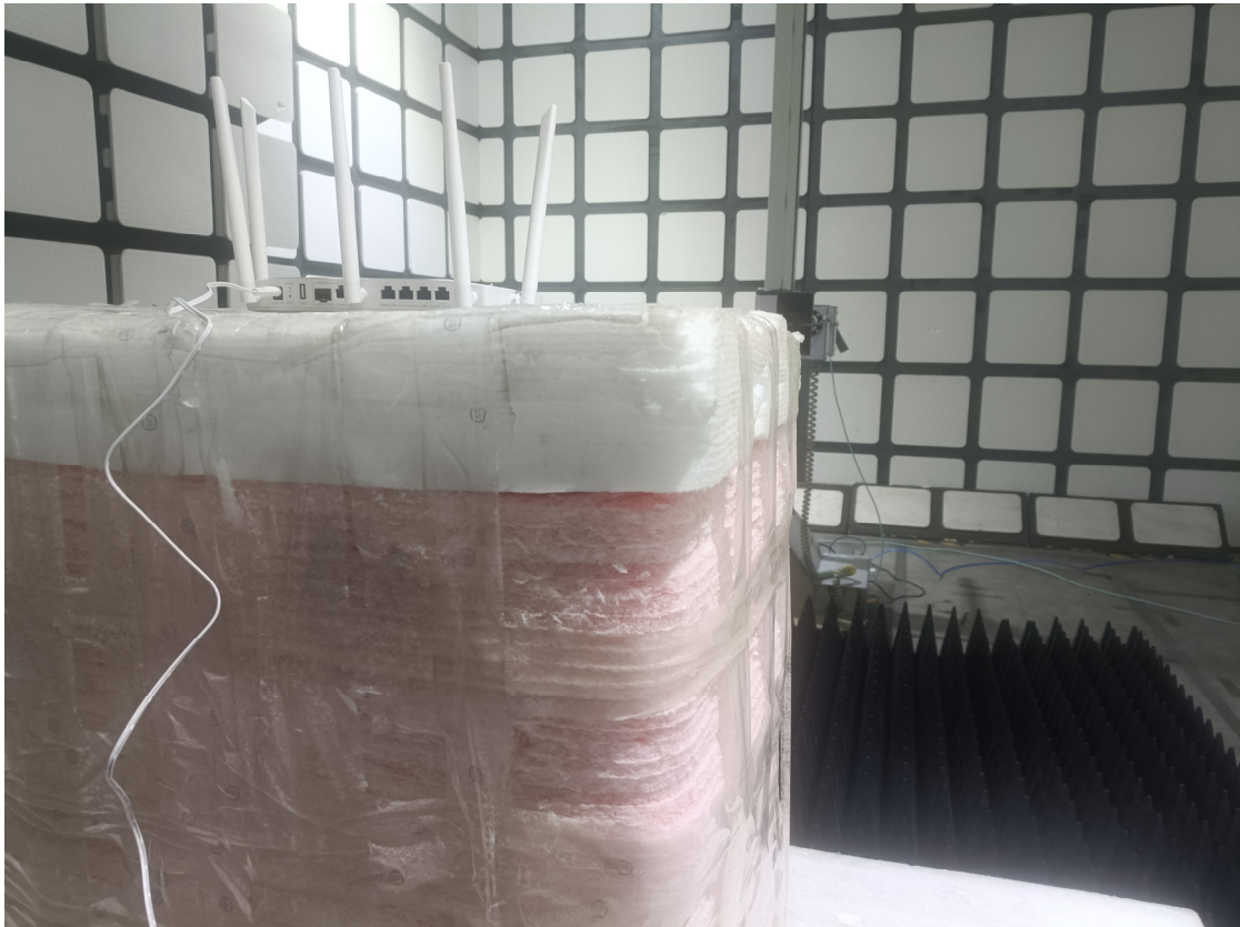
Radiated Emissions View (18-40 GHz)
