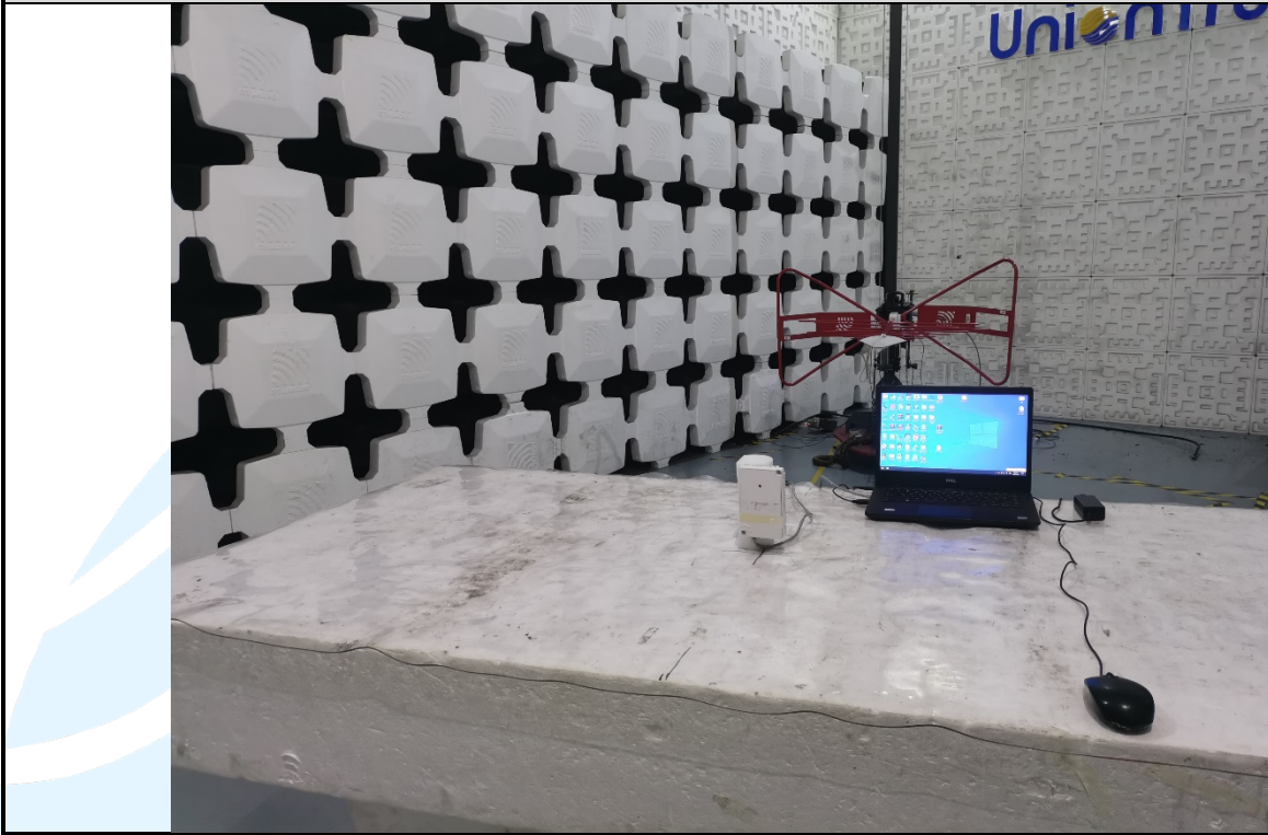
Radiated emission Test Setup (30 MHz~1 GHz)
