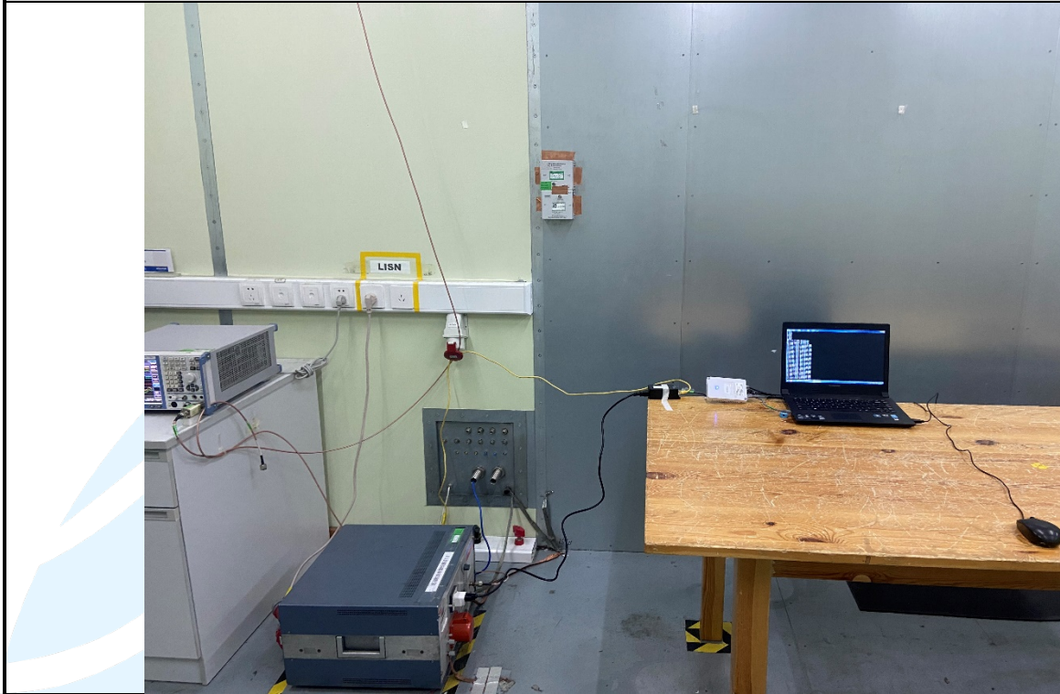
Conducted Emission Test Setup
