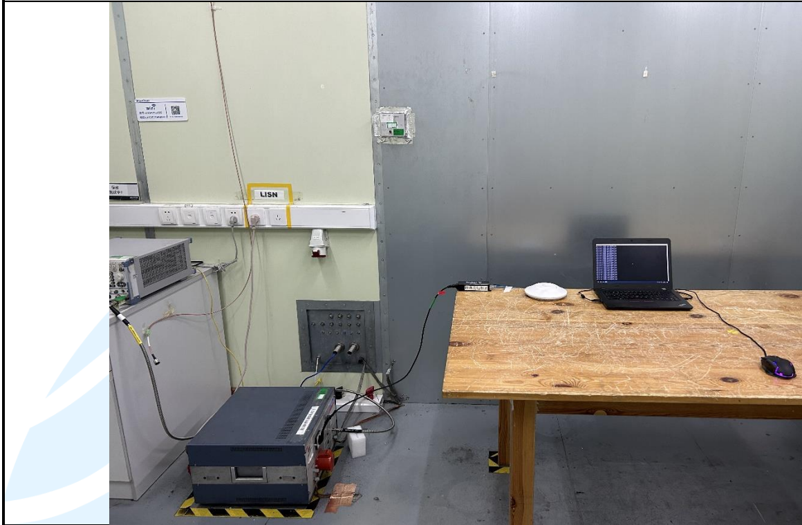
Conducted Emission Test Setup
