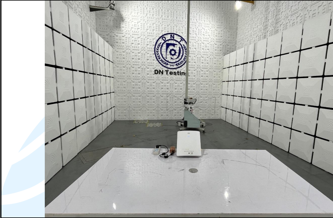
Radiated emission Test Setup (30 MHz~1 GHz)
