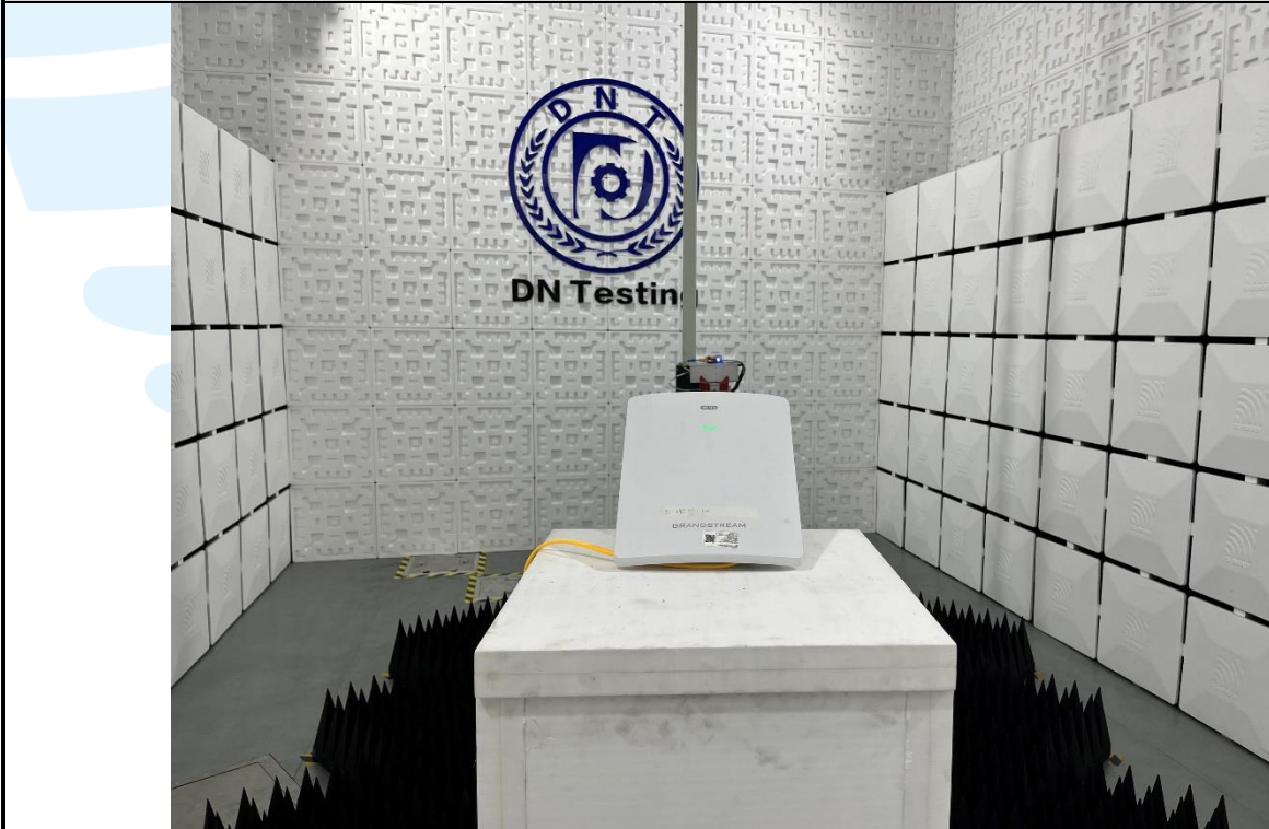
Radiated emission Test Setup (Above 1 GHz)
