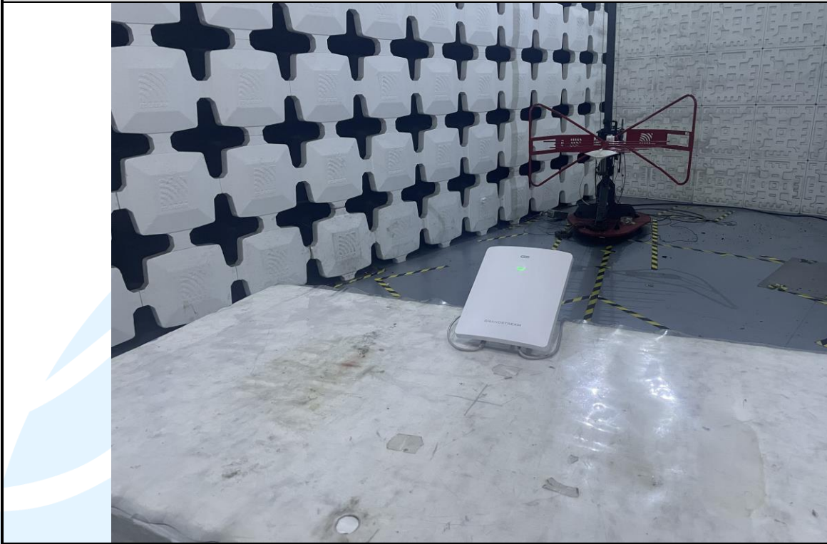
Radiated emission Test Setup-1 (30 MHz~1 GHz)
