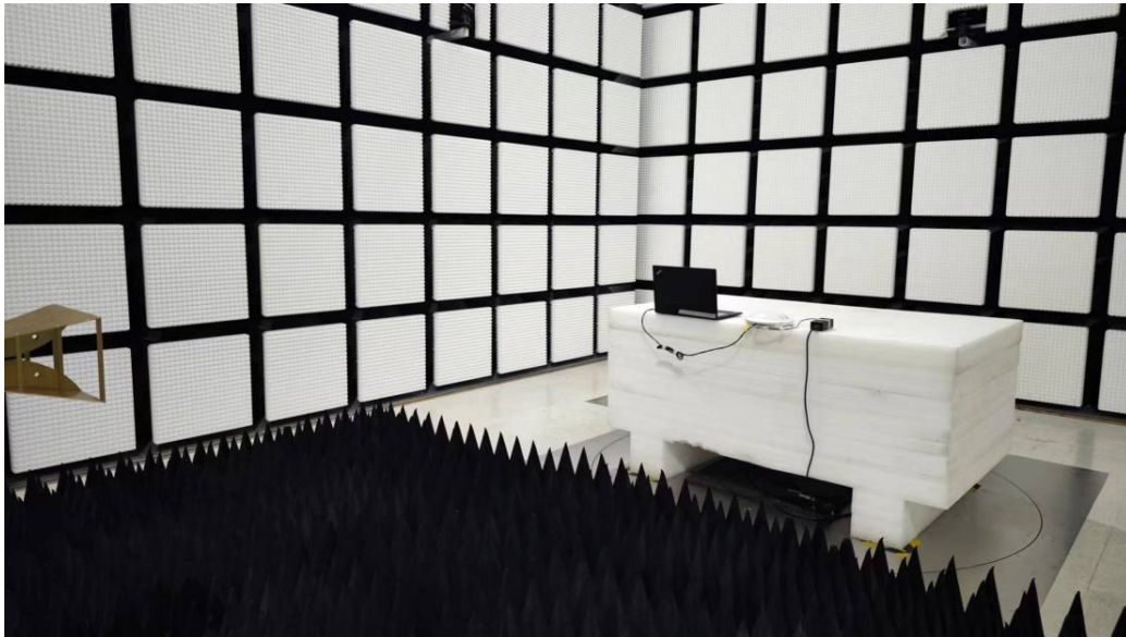
Radiated Emissions Above 1G rear View
