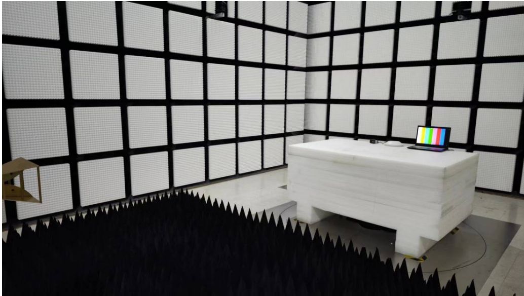
Radiated Emissions Above 1G rear View
