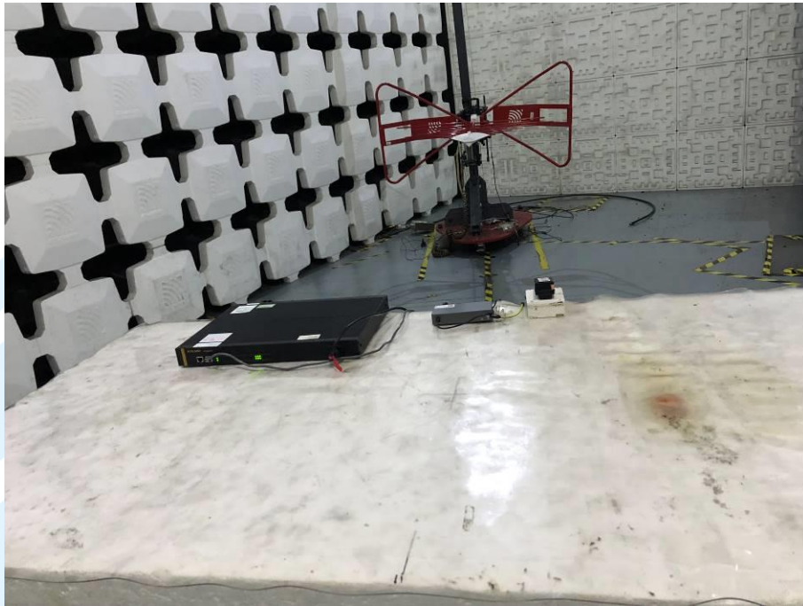
Radiated emission Test Setup-1 (30 MHz~1 GHz)
