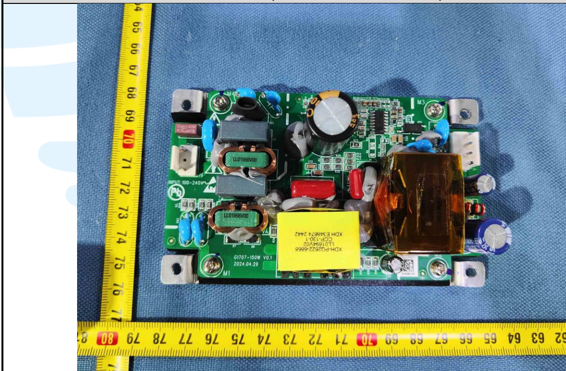
EUT Photo(Power board: G1707-150W)
