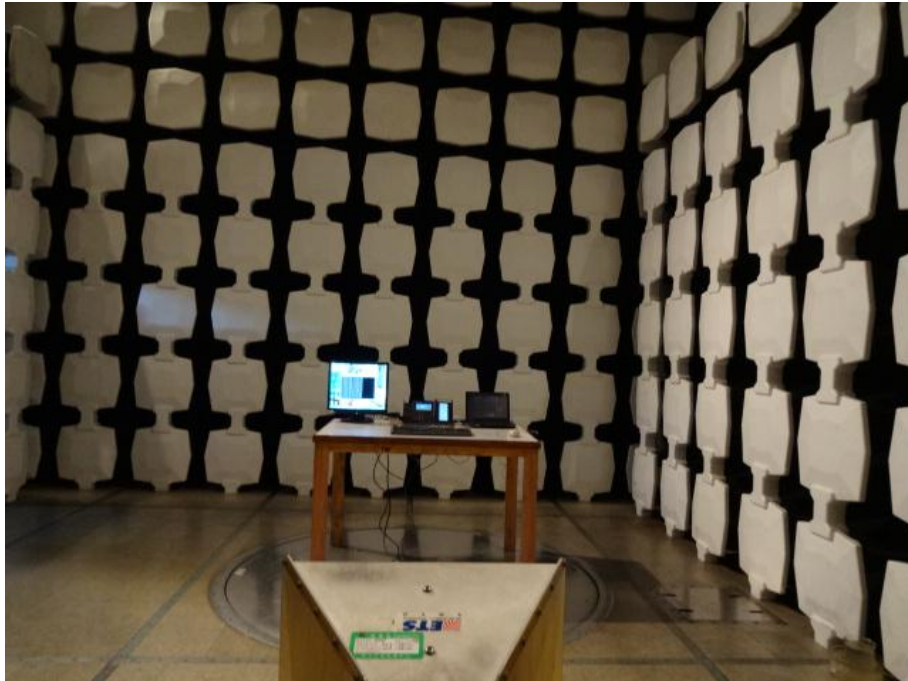
Radiated Emission Test Set-up (Above 1GHz)
