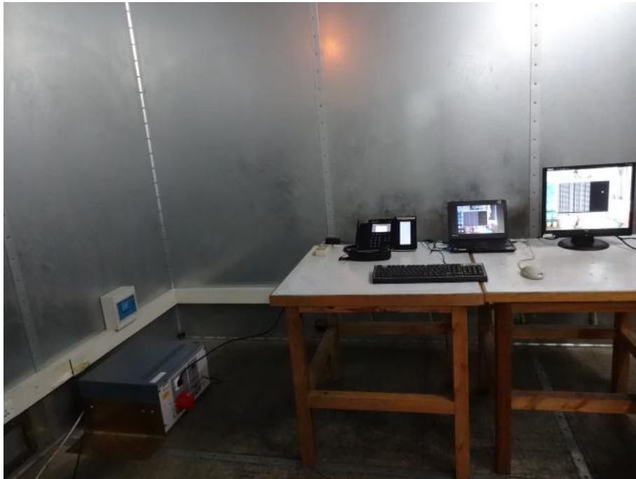
Conducted Emission Test Set-up –front view
