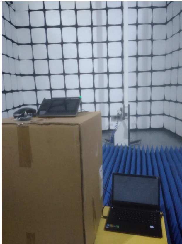
Radiated Emission test view (Frequency above 1GHz)
