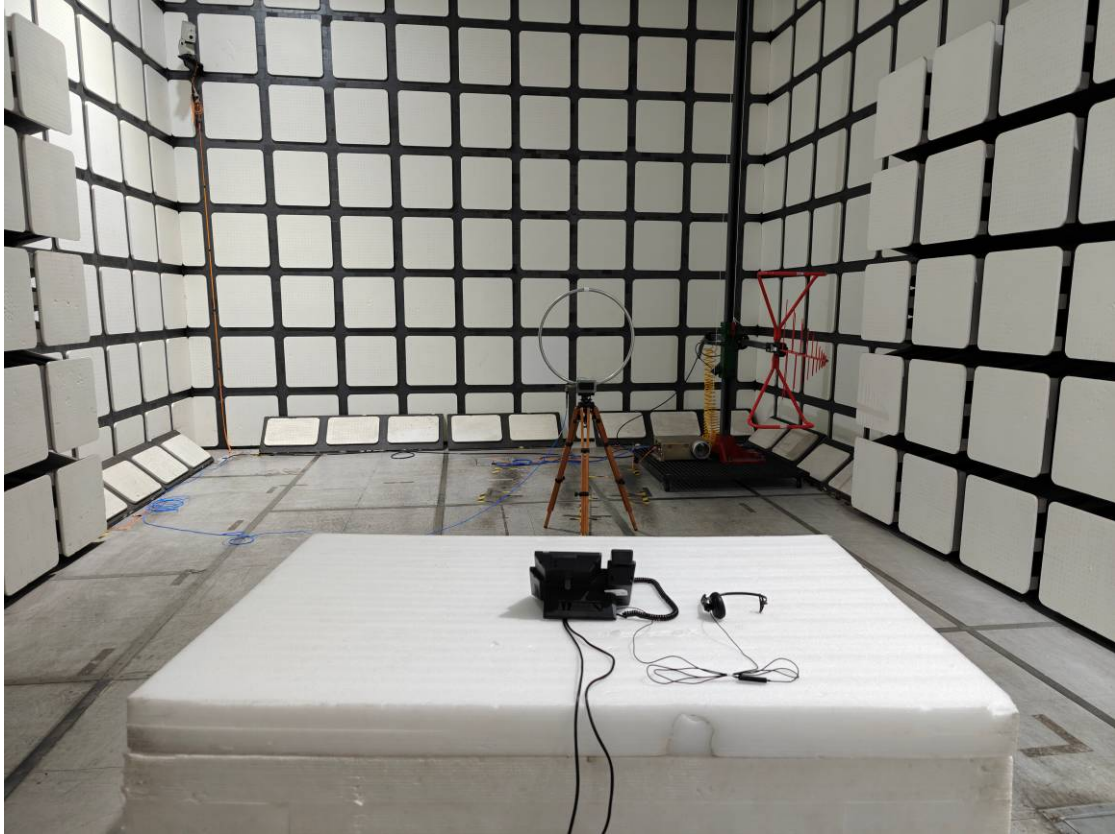
Radiated Emissions View (Below 1 GHz)_POE
