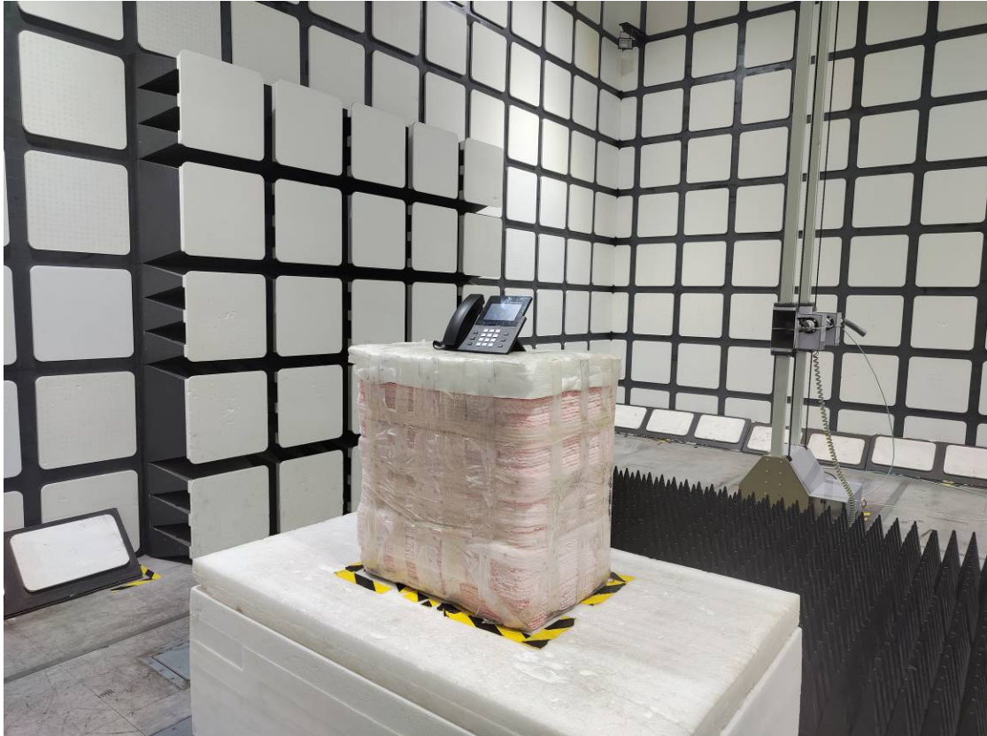
Radiated Emissions View (1-18 GHz)
