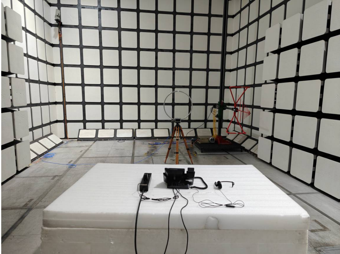
Radiated Emissions View (Below 1 GHz)_Adapter
