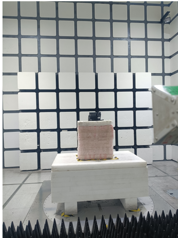
Radiated Emissions View (18-25GHz)
