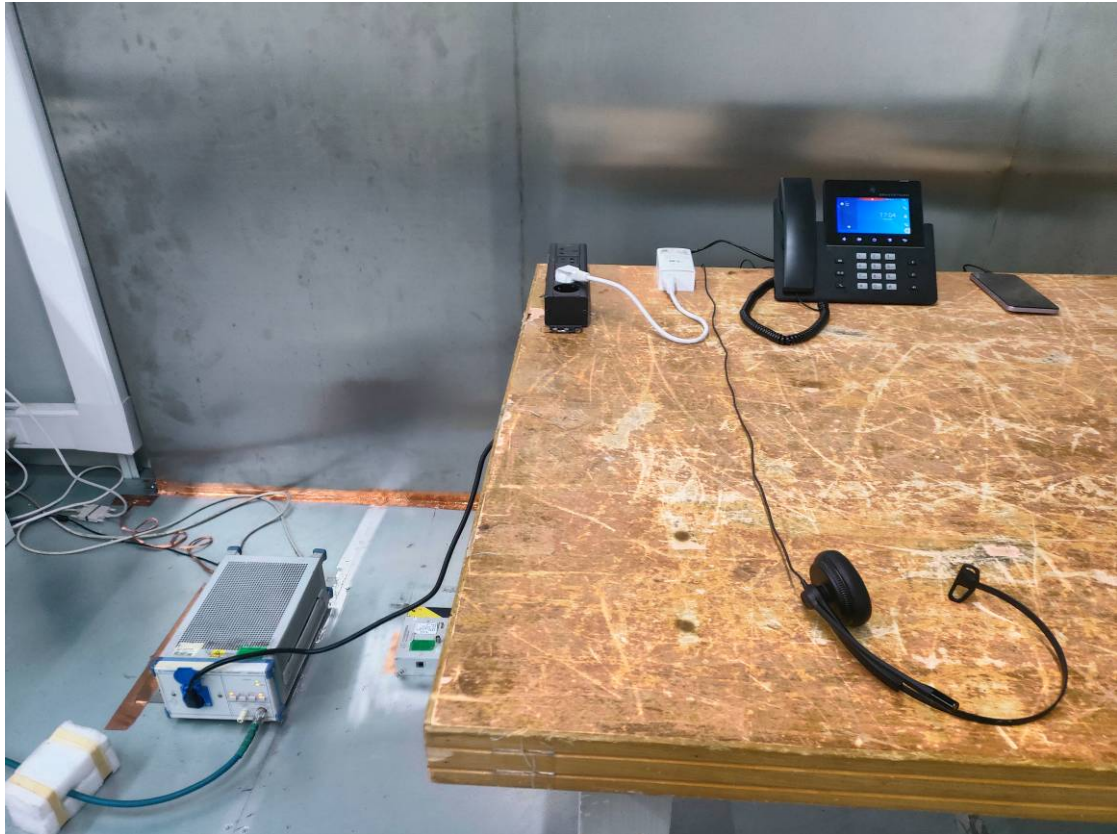
Conducted Emissions - Side View_POE
