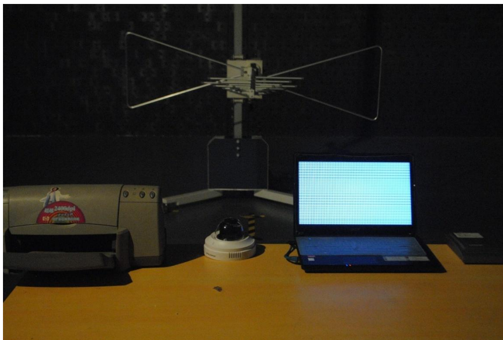
Radiated Emission test view (Frequency above 1GHz)
