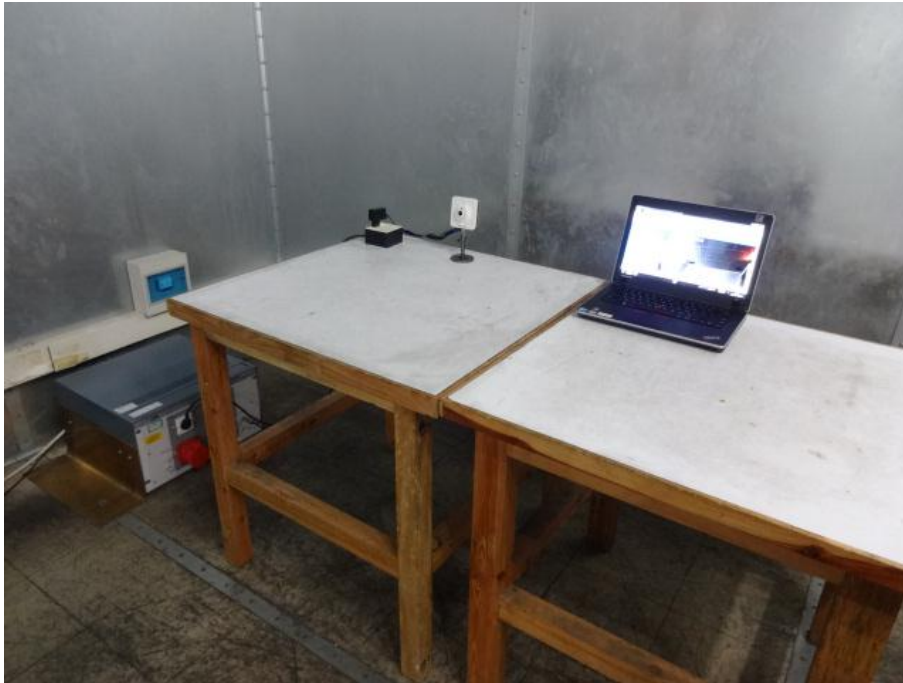
Conducted Emission Test Set-up –Front View
