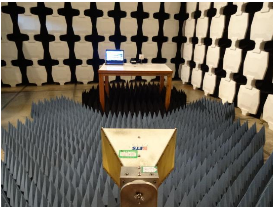
Radiated Emission Test Set-up (Above 1GHz)
