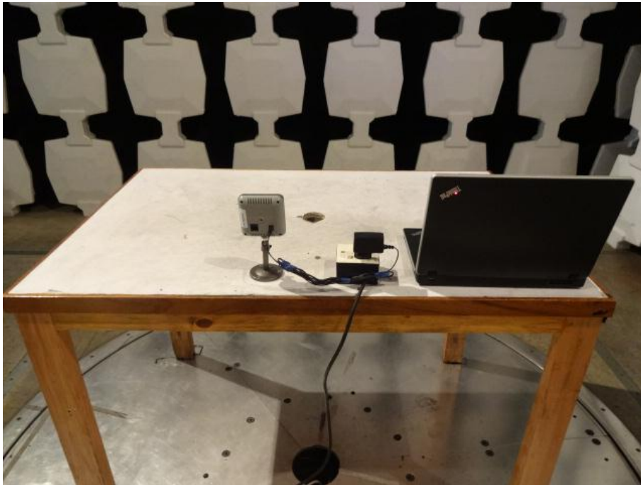
Radiated Emission Test Set-up (Rear View)
