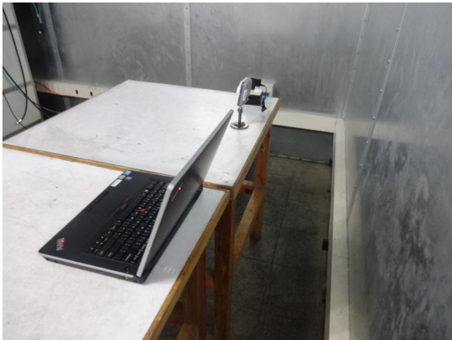
Conducted Emission Test Set-up-Rear View
