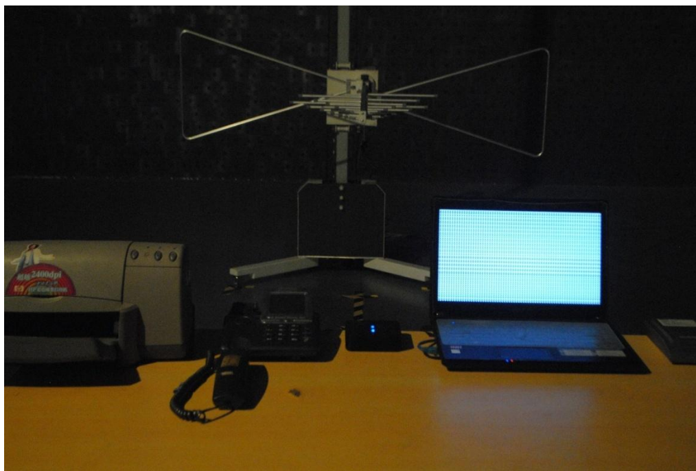
Radiated Emission test view (From 30MHz to 1GHz)
