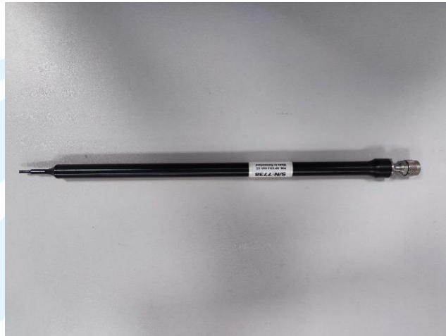
Speag COMOSAR Dosimetric E field Dipole
