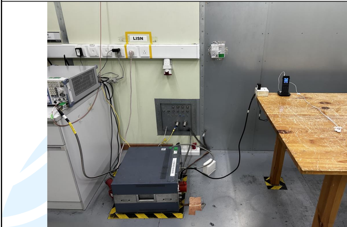
Conducted Emission Test Setup
