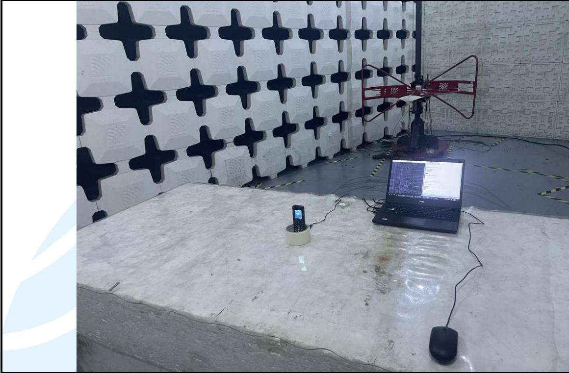
Radiated emission Test Setup (30 MHz~1 GHz)
