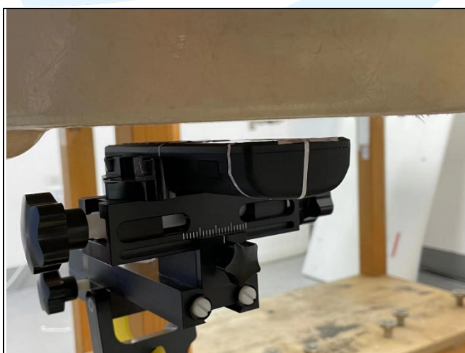
Front Face of EUT with 1.0 cm Gap
