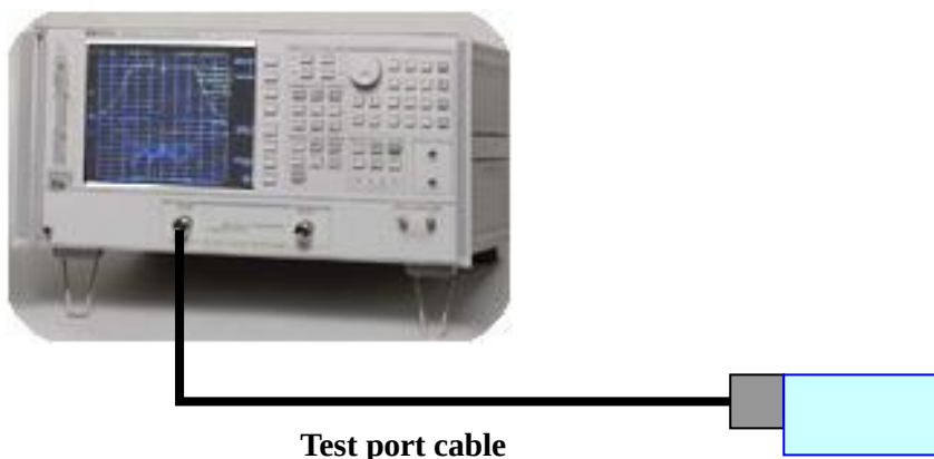
Figure 1. The schematic diagram for measuring VSWR
