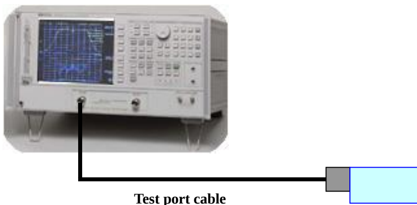
Figure 1. The schematic diagram for measuring VSWR
