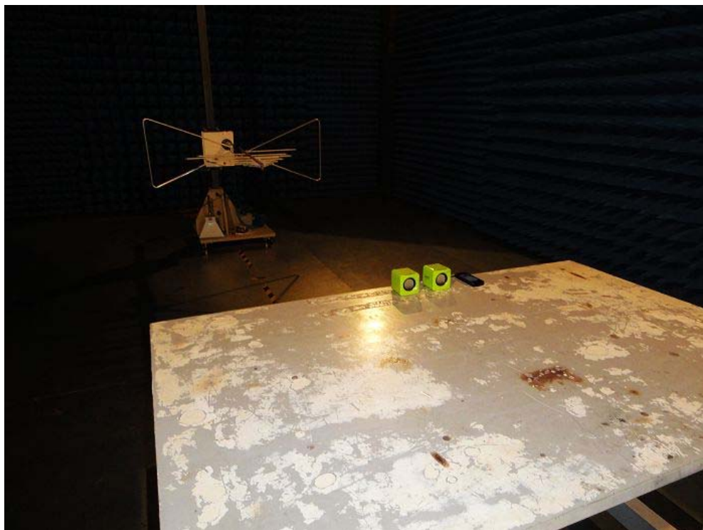
Radiated Emission Test Setup:
