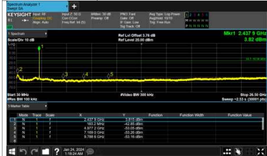
Tx. Spurious NVNT b 2462MHz Ant2 Ref
