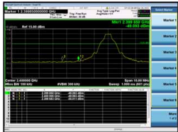
GFSK LOW CHANNEL, BAND EDGE
