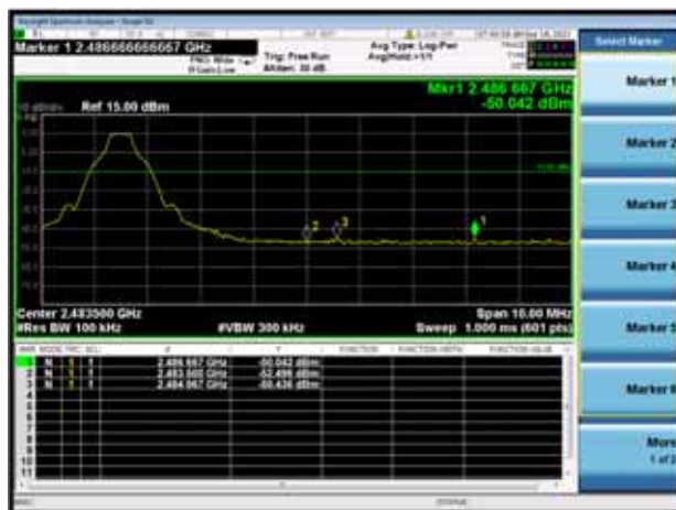
GFSK HIGH CHANNEL, BAND EDGE
