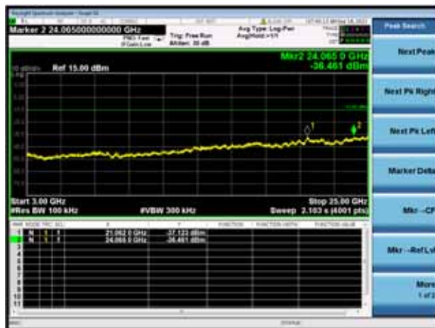
GFSK HIGH CHANNEL, SPURIOUS 3 GHz ~ 25 GHz
