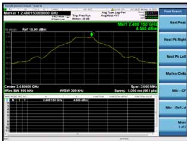
GFSK HIGH CHANNEL, CARRIER LEVEL
