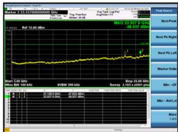
GFSK LOW CHANNEL, SPURIOUS 3 GHz ~ 25 GHz
