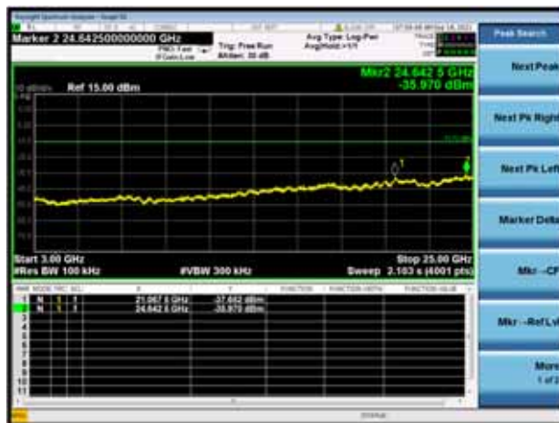
8-DPSK MIDDLE CHANNEL, SPURIOUS 3 GHz ~ 25 GHz
