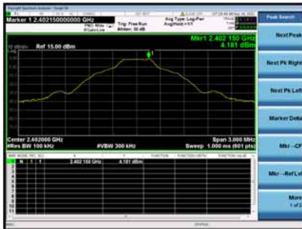
GFSK LOW CHANNEL, CARRIER LEVEL
