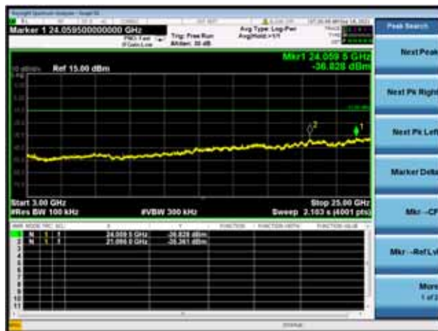
GFSK MIDDLE CHANNEL, SPURIOUS 3 GHz ~ 25 GHz
