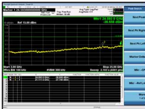
8-DPSK HIGH CHANNEL, SPURIOUS 3 GHz ~ 25 GHz
