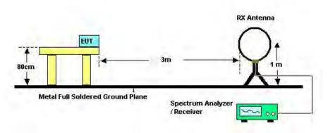
For Radiated Emissions: 30MHz~1GHz
