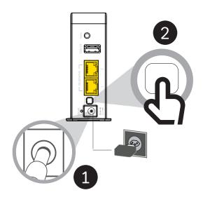
Connect the additional Air 4920 to electric power (1) and power it up by pressing the power button (2) as shown left.
