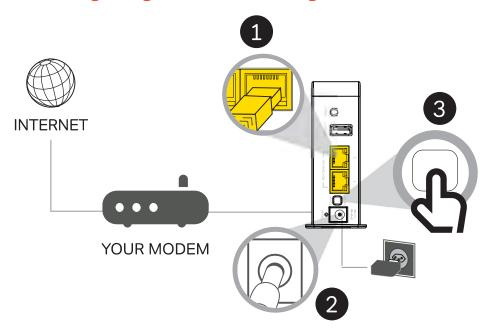
Connect the Air 4920 to Internet gateway via Ethernet Cable (1) and electric power (2) as show above and power it up by pressing the power button (3).
