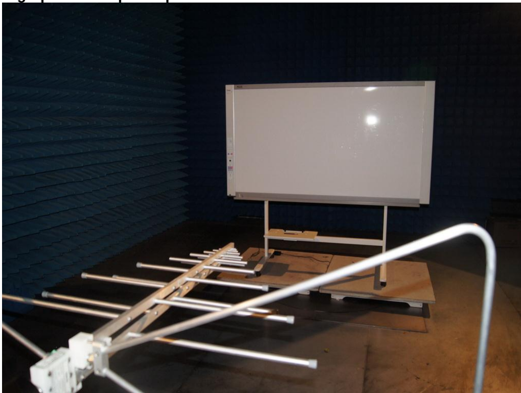
Photograph 4: Set-up for Spurious Emissions for 30 - 1000MHz
