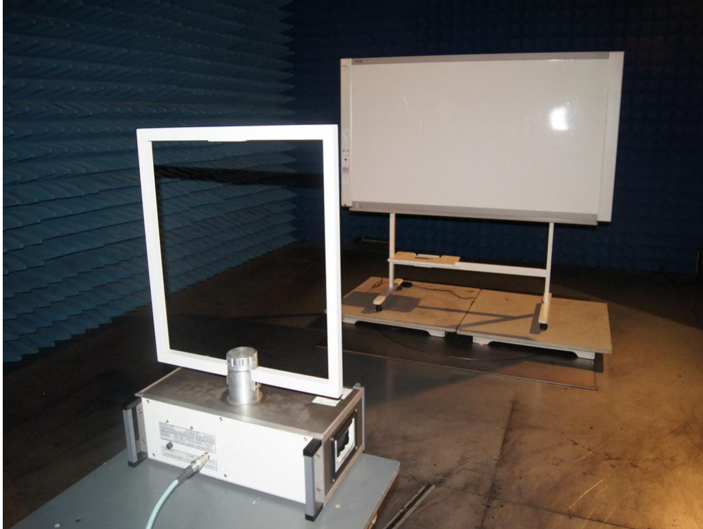
Photograph 4: Set-up for Spurious Emissions for 30 - 1000MHz
