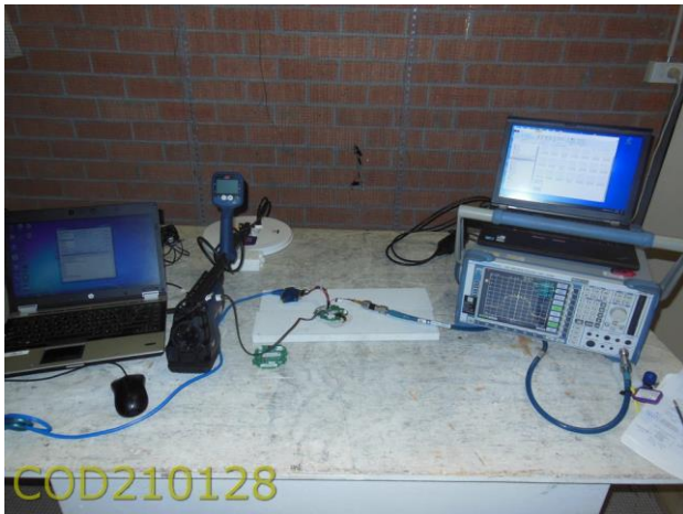
View Bench Test RF Port Conducted
