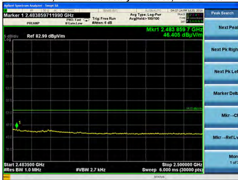
Channel 39, Side Orientation, Antenna Vertically Polarized, 2483.5-2500 MHz, Average at 3m
