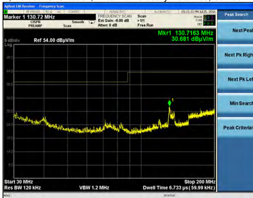
Channel 1, Vertical Orientation, Antenna Vertically Polarized, 30-200 MHz, at 3m
