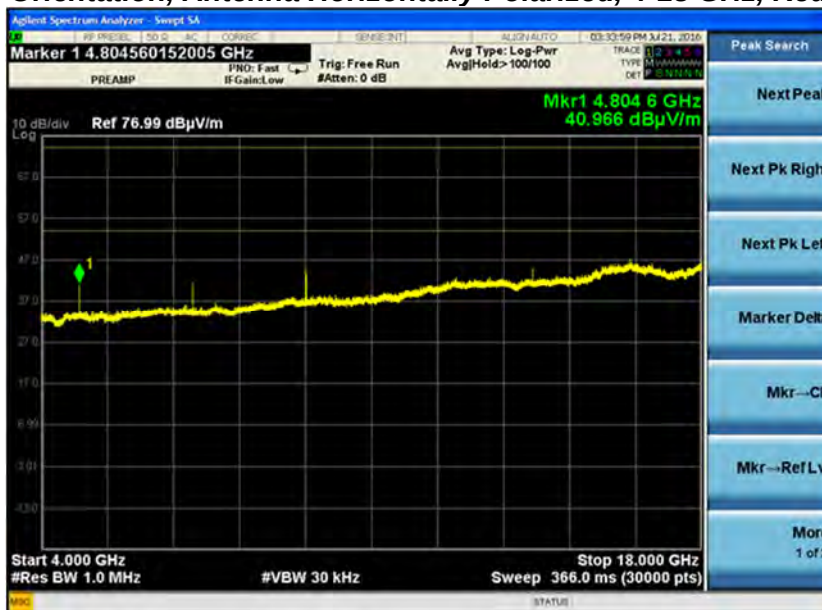
Channel 0, Side Orientation, Antenna Horizontally Polarized, 4-18 GHz, Reduced VBW at 3m
