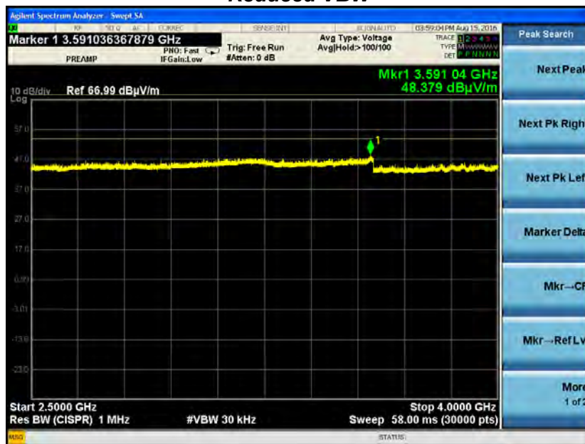
Channel 39, Vertical Orientation, Antenna Vertically Polarized, 2500 MHz to 4000 MHz, Reduced VBW
