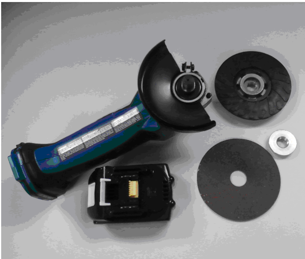
Figure 7. Assembling the Grinder
