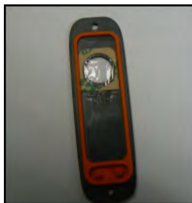
Figure 6. Measurement Window Replaced
