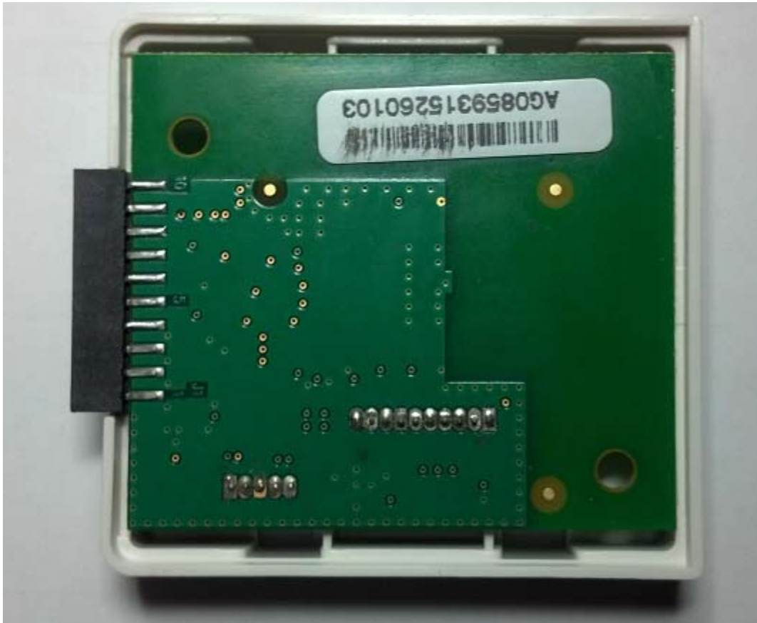
Rear of PCB showing Ground Plane
