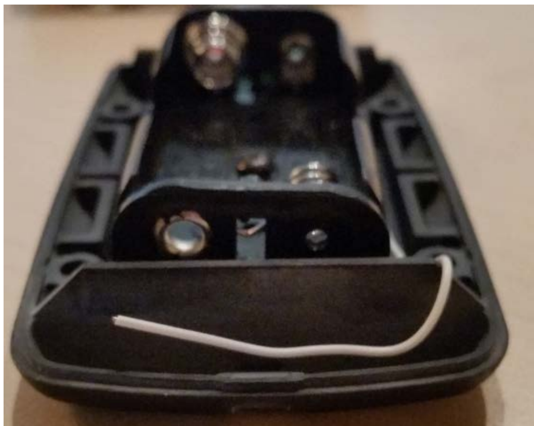
Fig. 6, Front of assembly showing antenna
