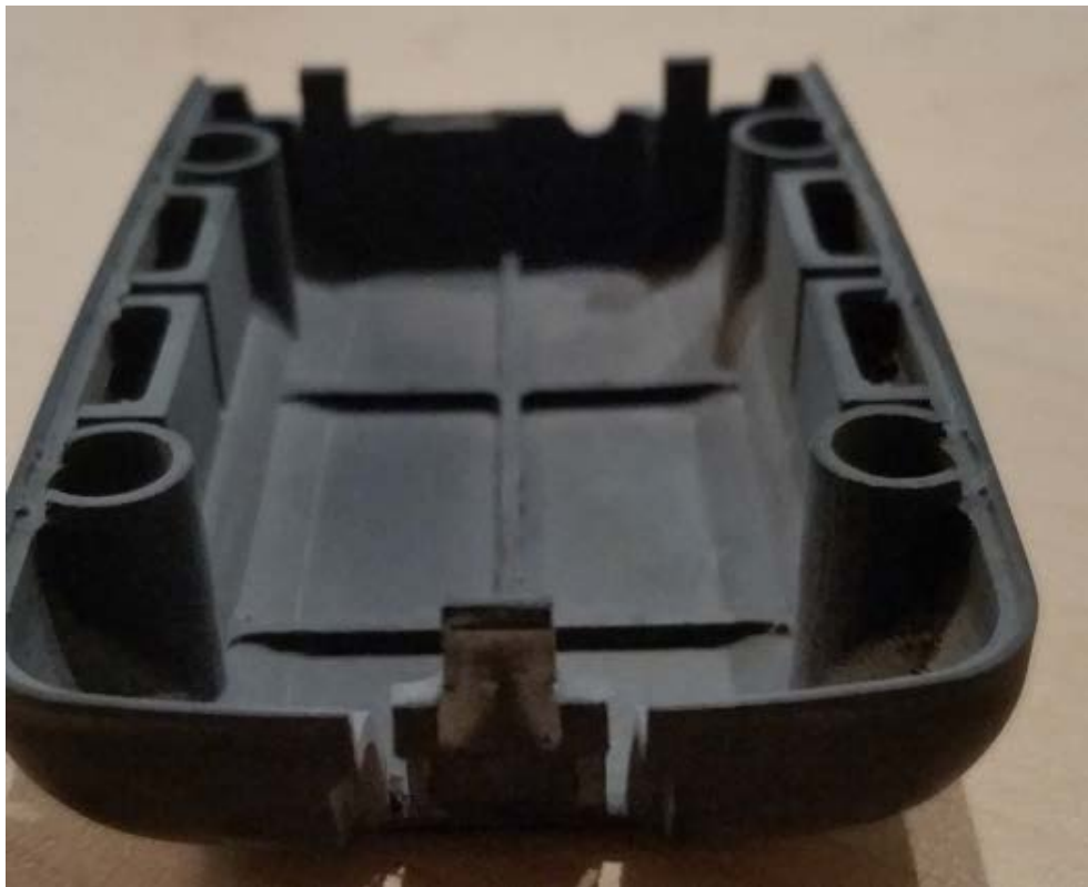
Fig 8. Bottom of enclosure with circuit board and battery compartment removed.
