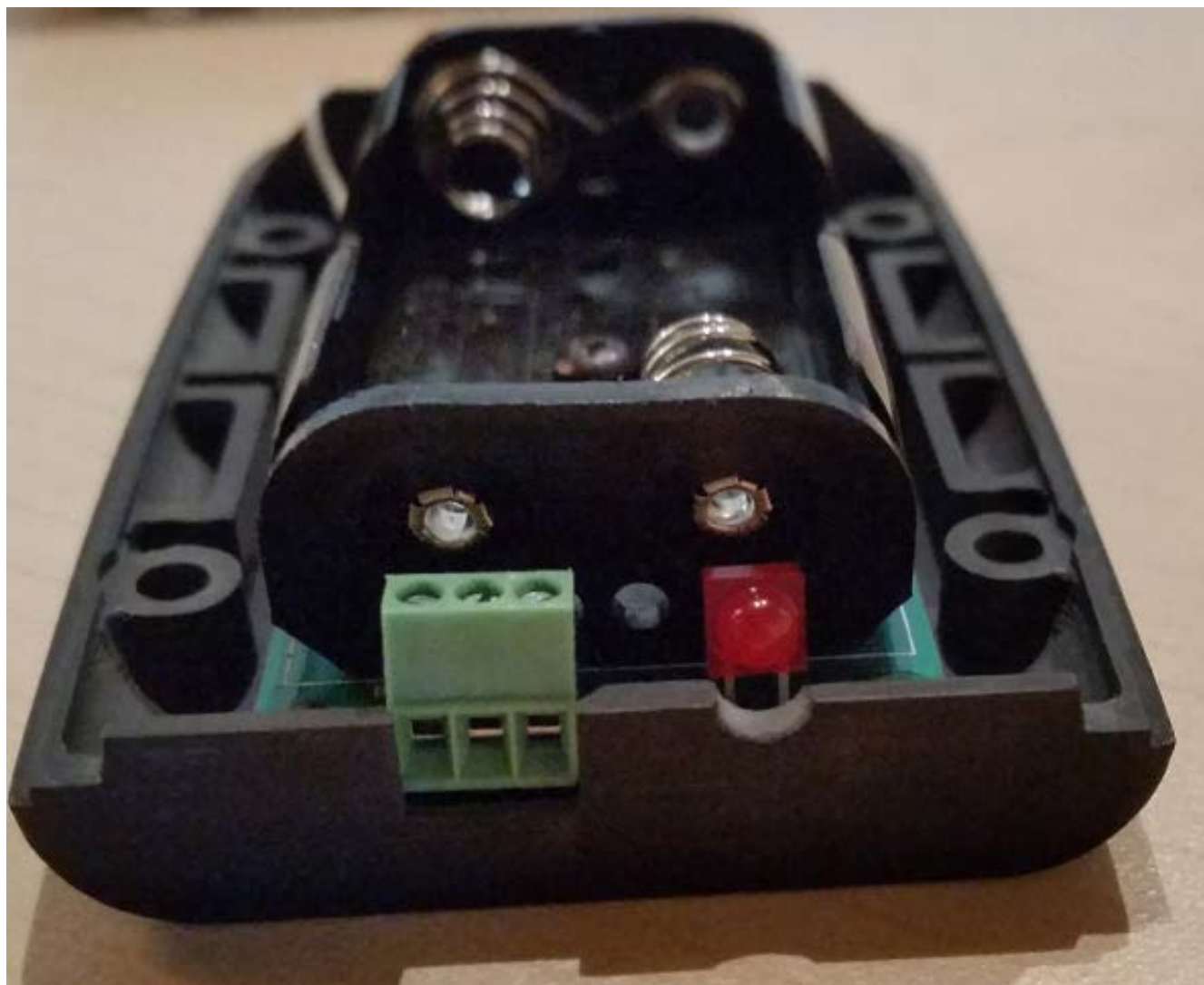
Fig 4. Rear assembly, showing the terminal block and LED
