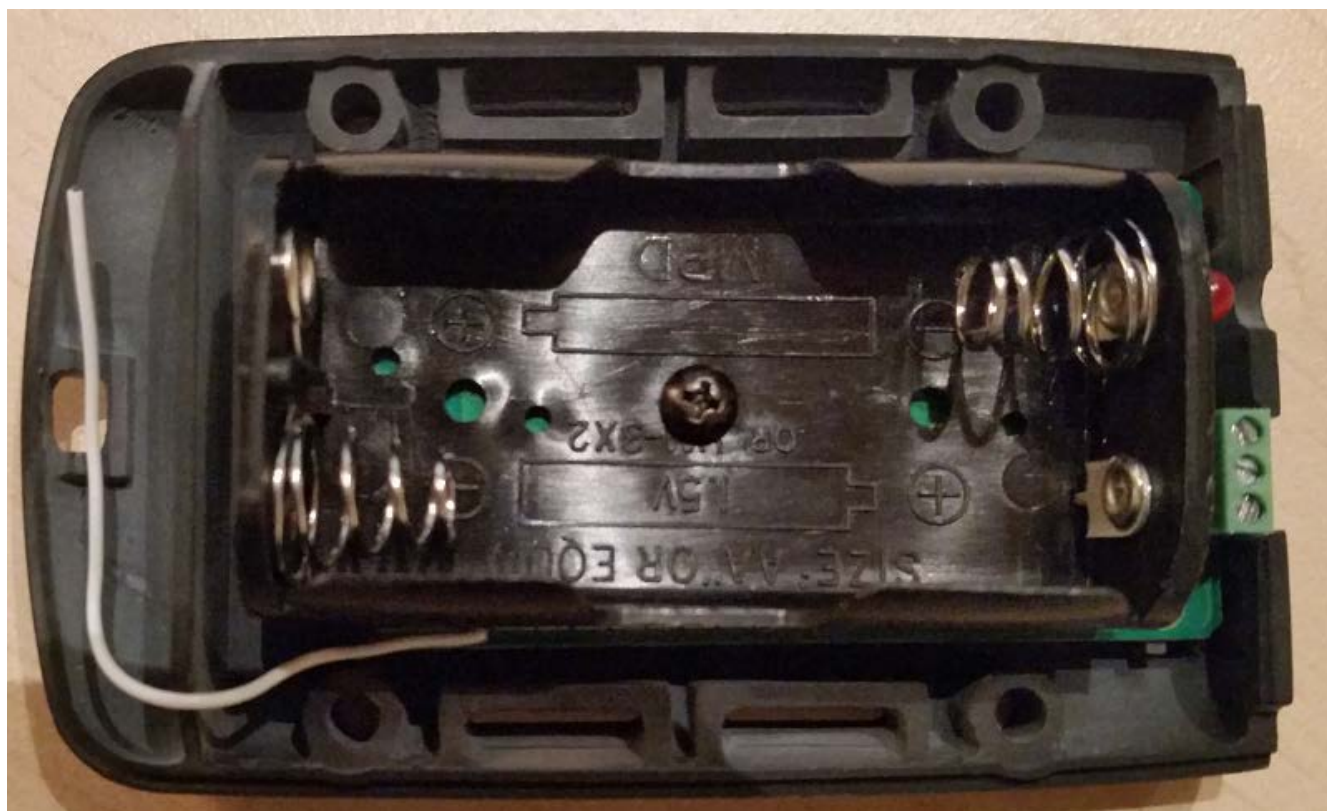
Fig 3. Close up of the Battery Compartment Left-hand side, showing the wire antenna placement.
