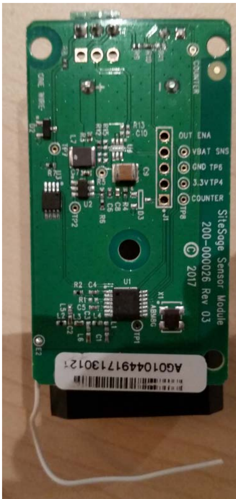
Fig. 11 PCB assembly from the bottom showing the surface mount components.
