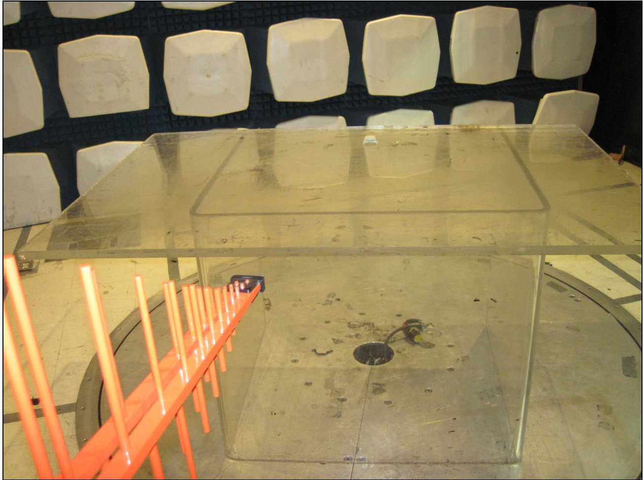
Photograph 2. RF Output Power, Test Setup
