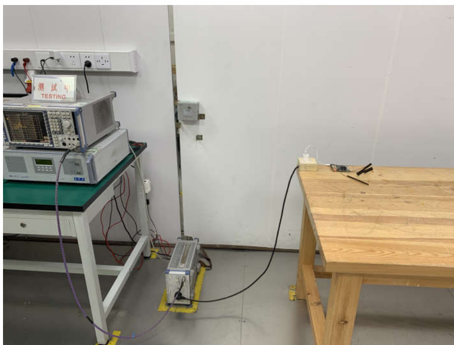
Conducted Emissions Test Setup
