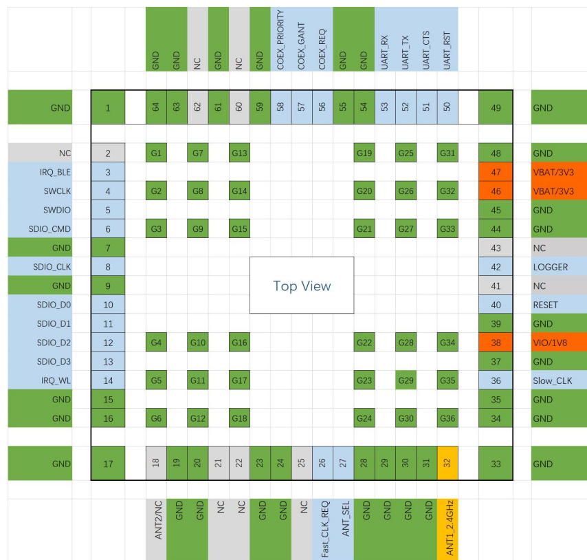
Figure 2-3. BM3301-1313 Module Pin arrangement
