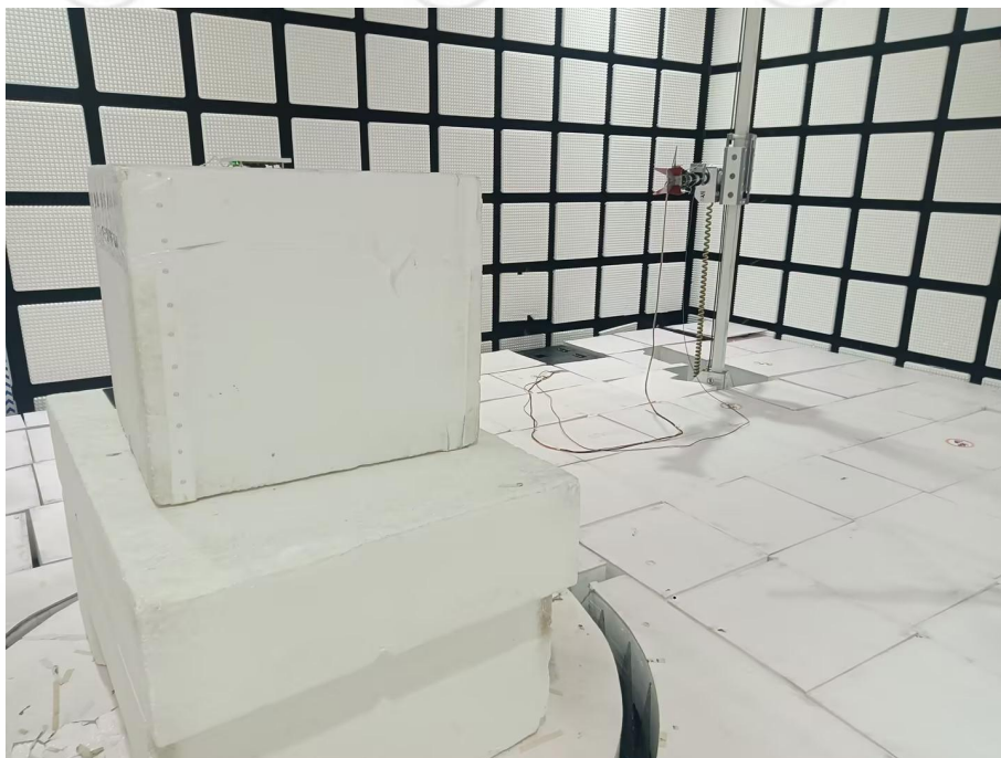
Radiated spurious emission Test Setup-3(Above 1GHz)
