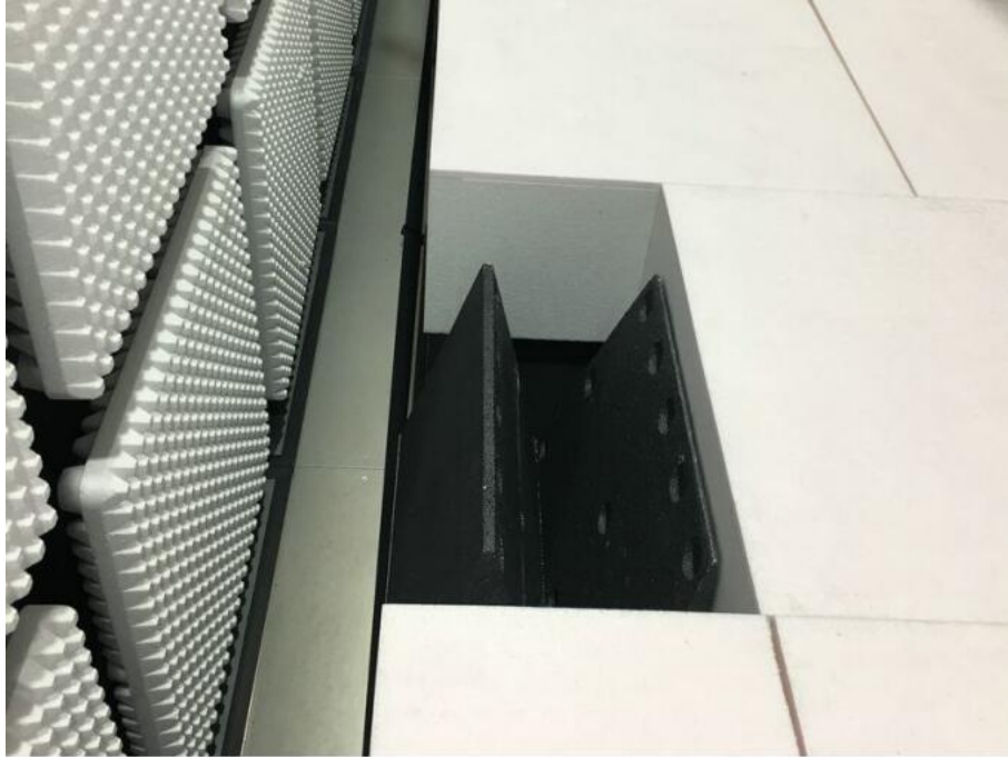
Radiated spurious emission Test Setup-5 There are absorbing materials under the ground.
