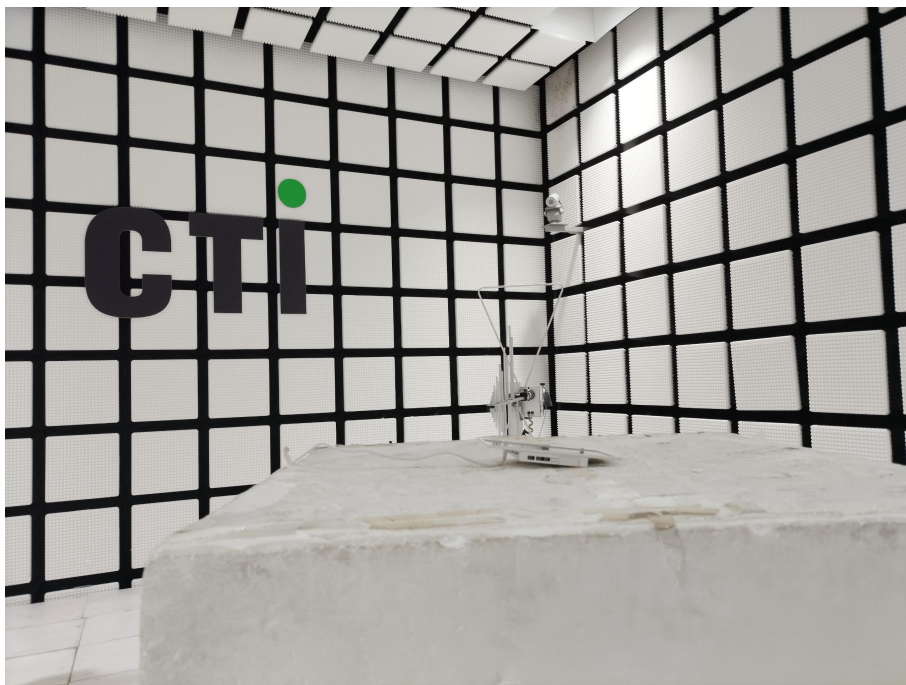
Radiated spurious emission Test Setup-1(Below 1GHz)
