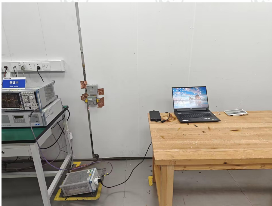
Conducted Emissions Test Setup
