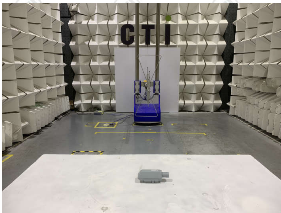
Radiated spurious emission Test Setup-1(Below 1GHz)
