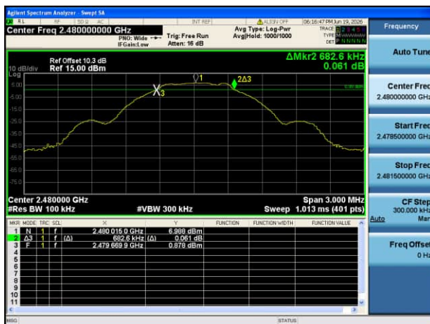
GFSK (BLE 1Mbps) HIGH CHANNEL
