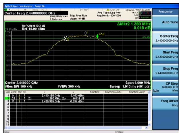
GFSK (BLE 2Mbps) MIDDLE CHANNEL
