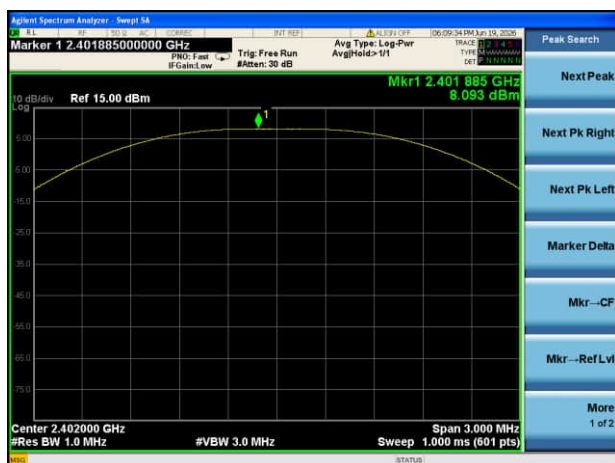
GFSK (BLE 1Mbps) LOW CHANNEL
