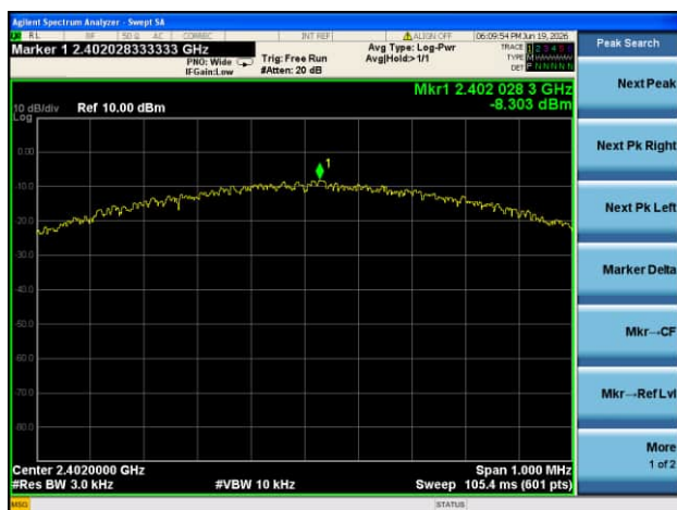
GFSK (BLE 1Mbps) LOW CHANNEL
