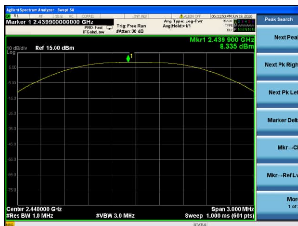
GFSK (BLE 1Mbps) MIDDLE CHANNEL
