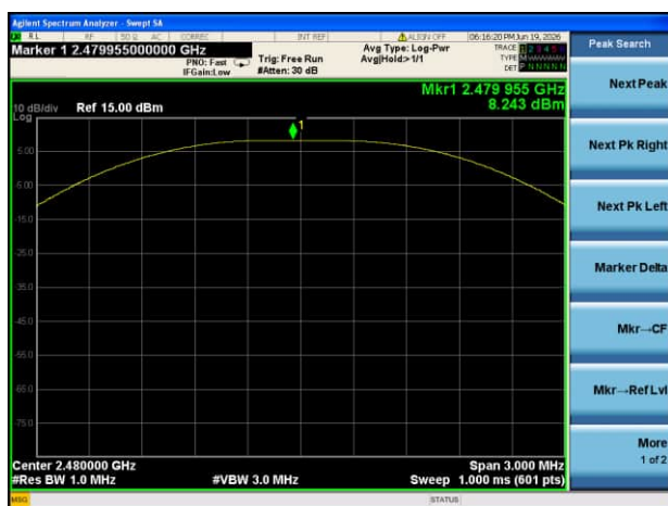
GFSK (BLE 1Mbps) HIGH CHANNEL
