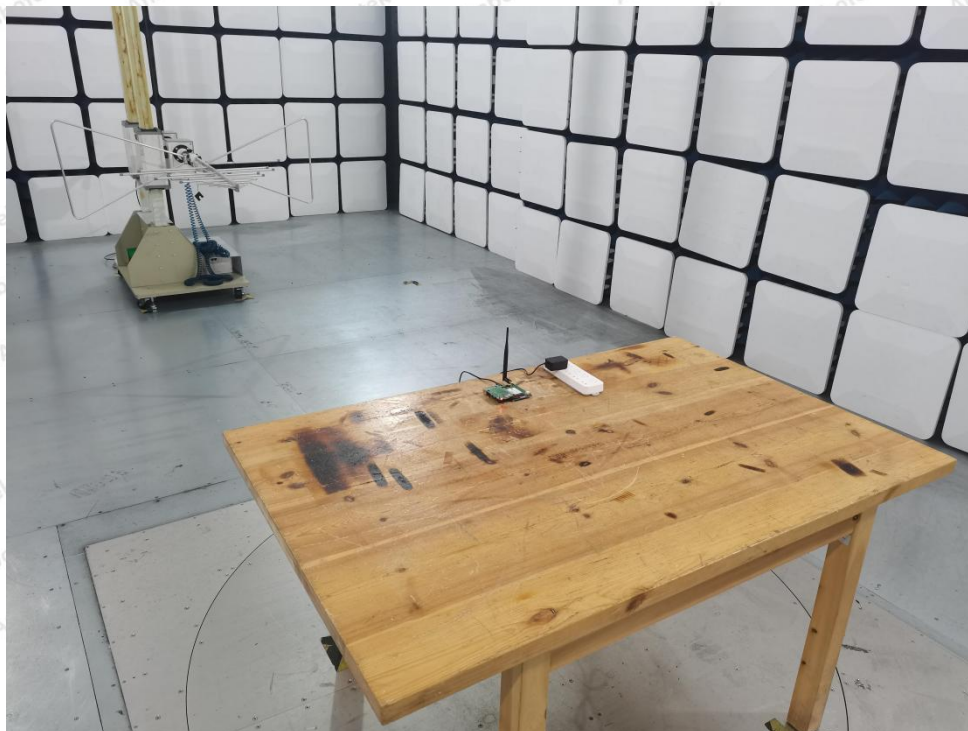
Photo of Radiation Emission Test
