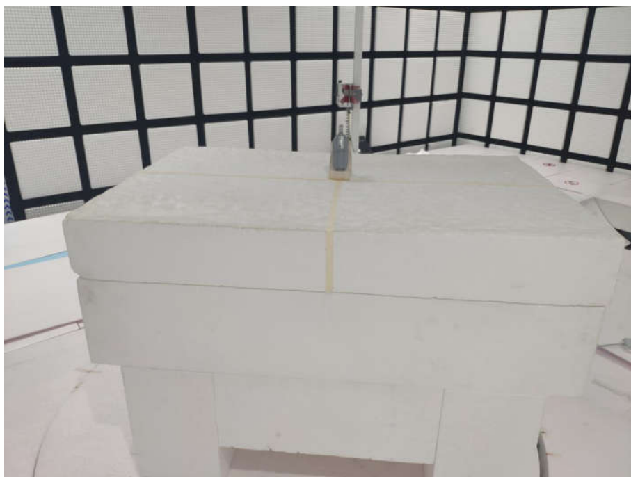
Radiated spurious emission Test Setup-1(Above 1GHz)
