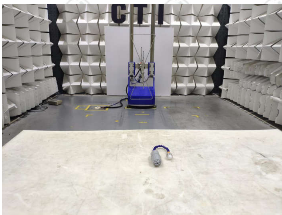
Radiated spurious emission Test Setup-3(Below 1GHz)
