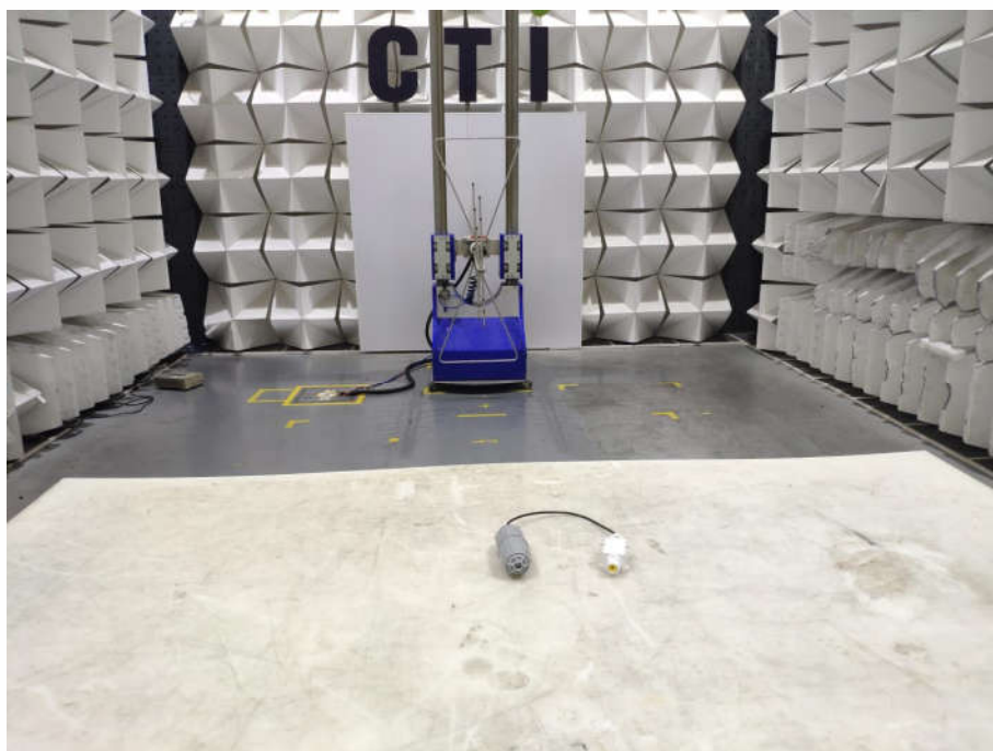
Radiated spurious emission Test Setup-4(Below 1GHz)
