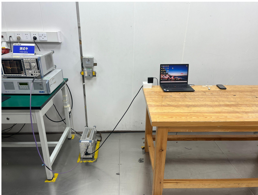
AC Power Line Conducted Emission Test Setup
