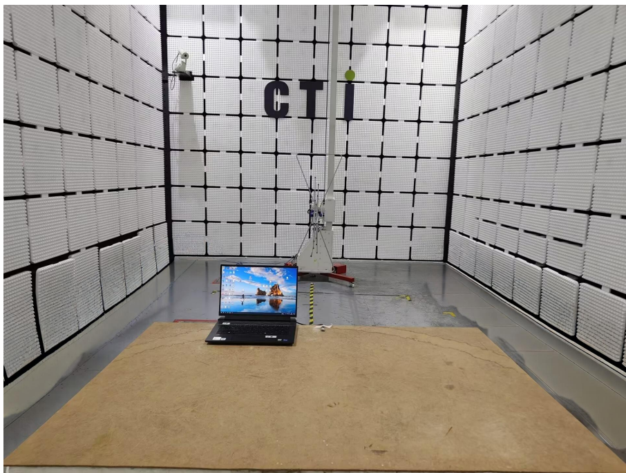
Radiated spurious emission Test Setup-1(Below 1GHz)
