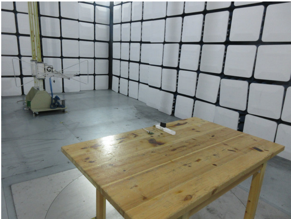
Photo of Radiation Emission Test
