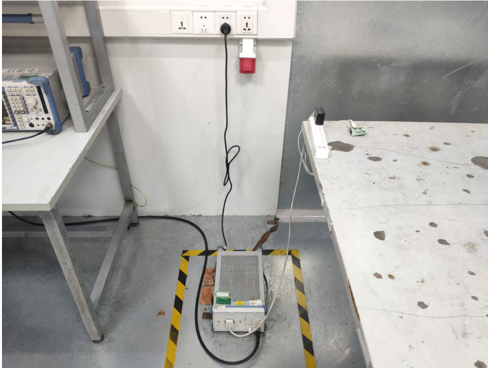
Photo of Power Line Conducted Emission Test
