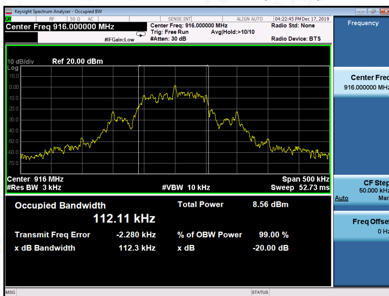
TEST PLOT OF BANDWIDTH (916MHz)
