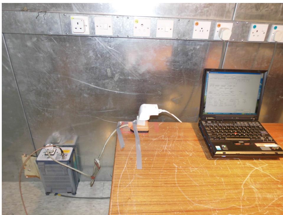
Set-up for AC Mains Conducted Emission
