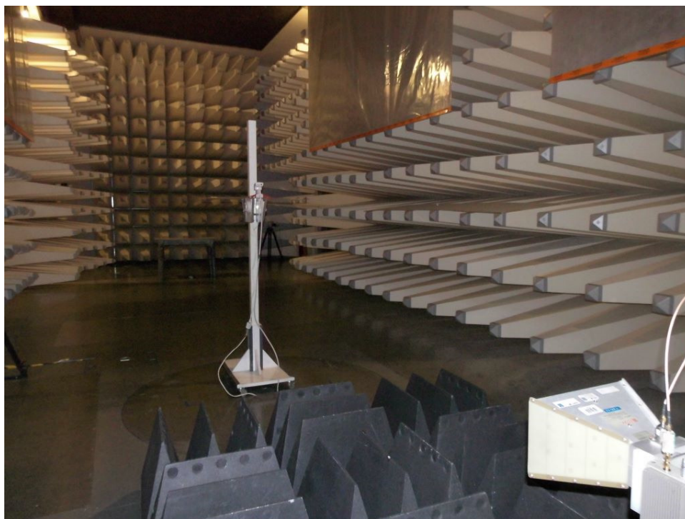
Set-up for Radiated Emission
