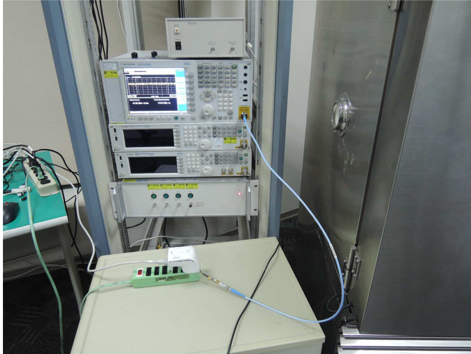
Photograph 4: Set-up for Conducted testing
