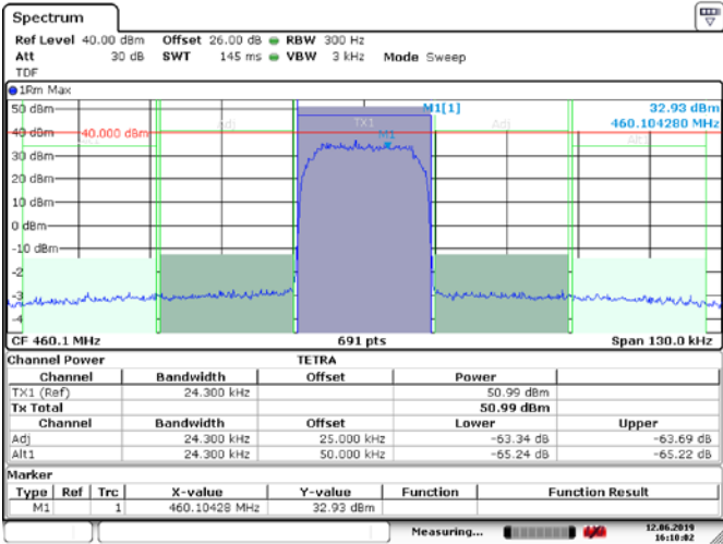
Figure 6.4-29: ACP, Tx @low channel of 460 MHz band, 25 W 0.35TETRA modulation
