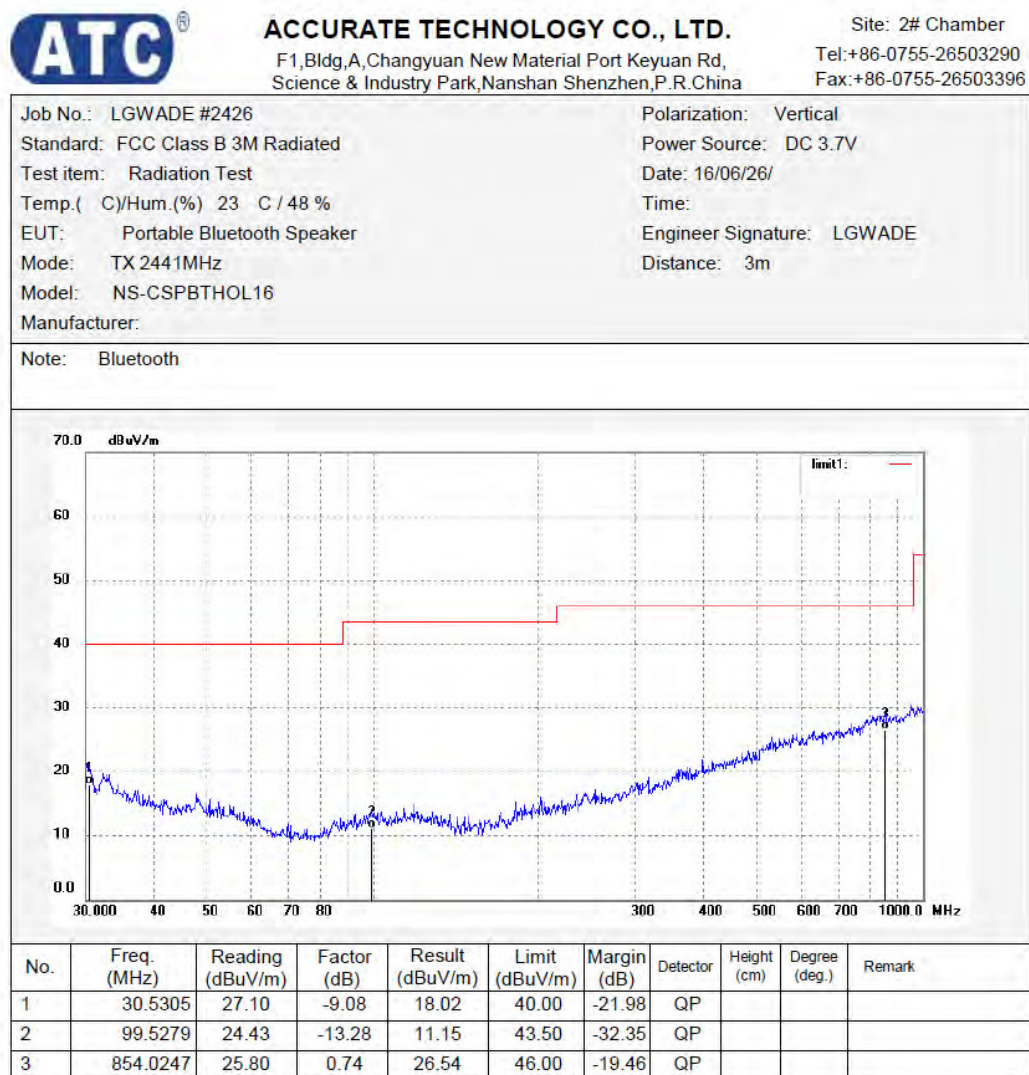
Figure 12: Test figure of spurious emissions, mode A.2, Vertical polarity (30MHz – 1GHz)
