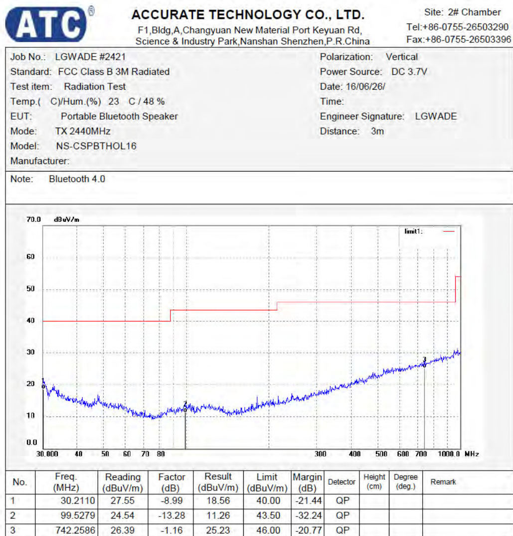
Figure 36: Test figure of spurious emissions, mode B.2, Vertical polarity (30MHz – 1GHz)
