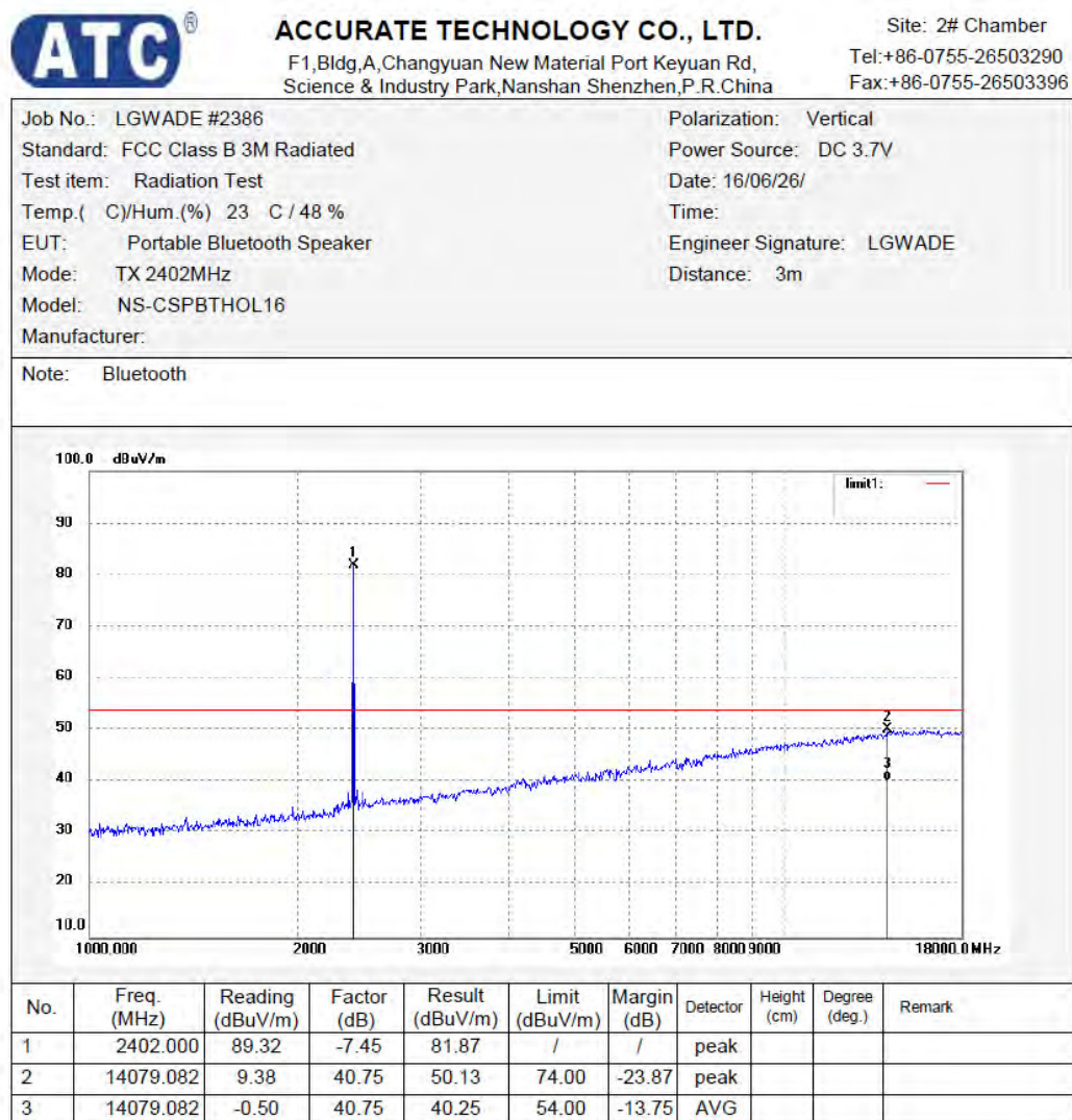
Figure 6: Test figure of spurious emissions, mode A.1, Vertical polarity (1GHz – 18GHz)
