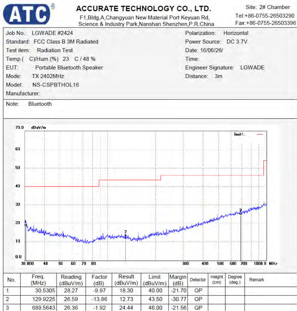
Figure 3: Test figure of spurious emissions, mode A.1, Horizontal polarity (30MHz – 1GHz)
