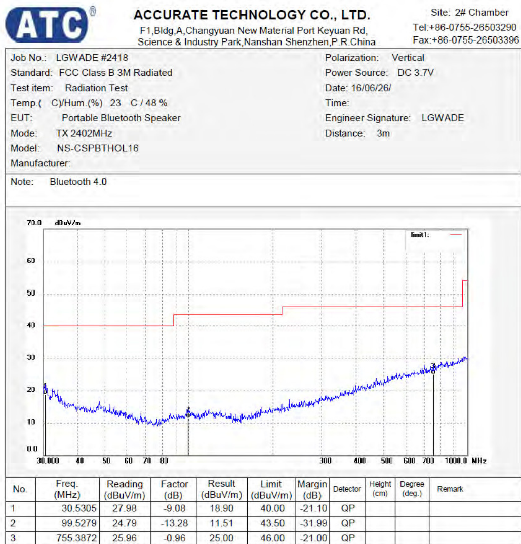
Figure 28: Test figure of spurious emissions, mode B.1, Vertical polarity (30MHz – 1GHz)
