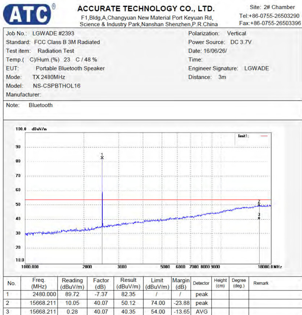
Figure 22: Test figure of spurious emissions, mode A.3, Vertical polarity (1GHz – 18GHz)
