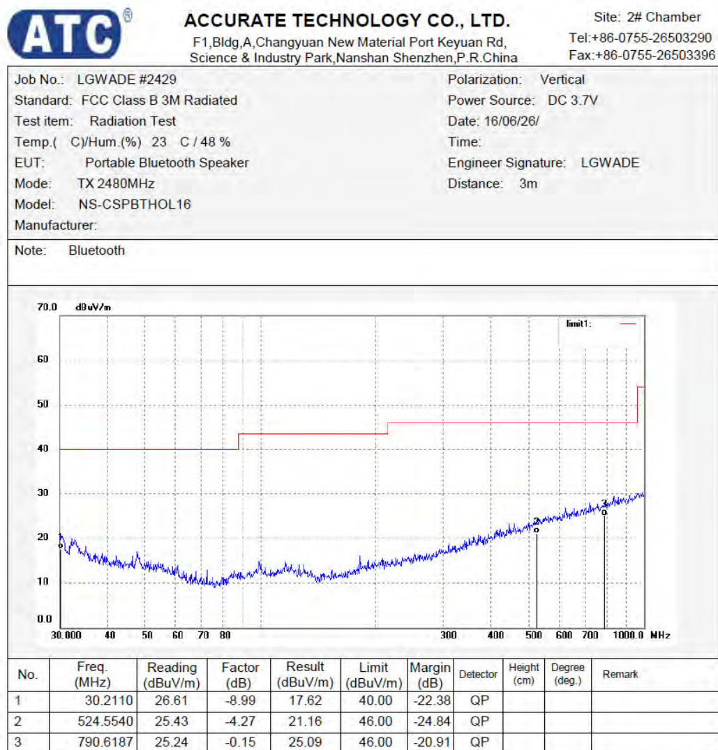
Figure 20: Test figure of spurious emissions, mode A.3, Vertical polarity (30MHz – 1GHz)
