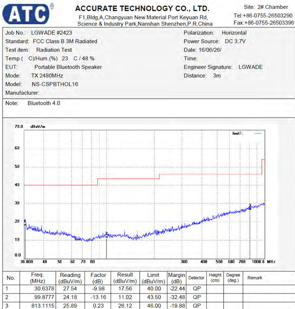
Figure 43: Test figure of spurious emissions, mode B.3, Horizontal polarity (30MHz – 1GHz)
