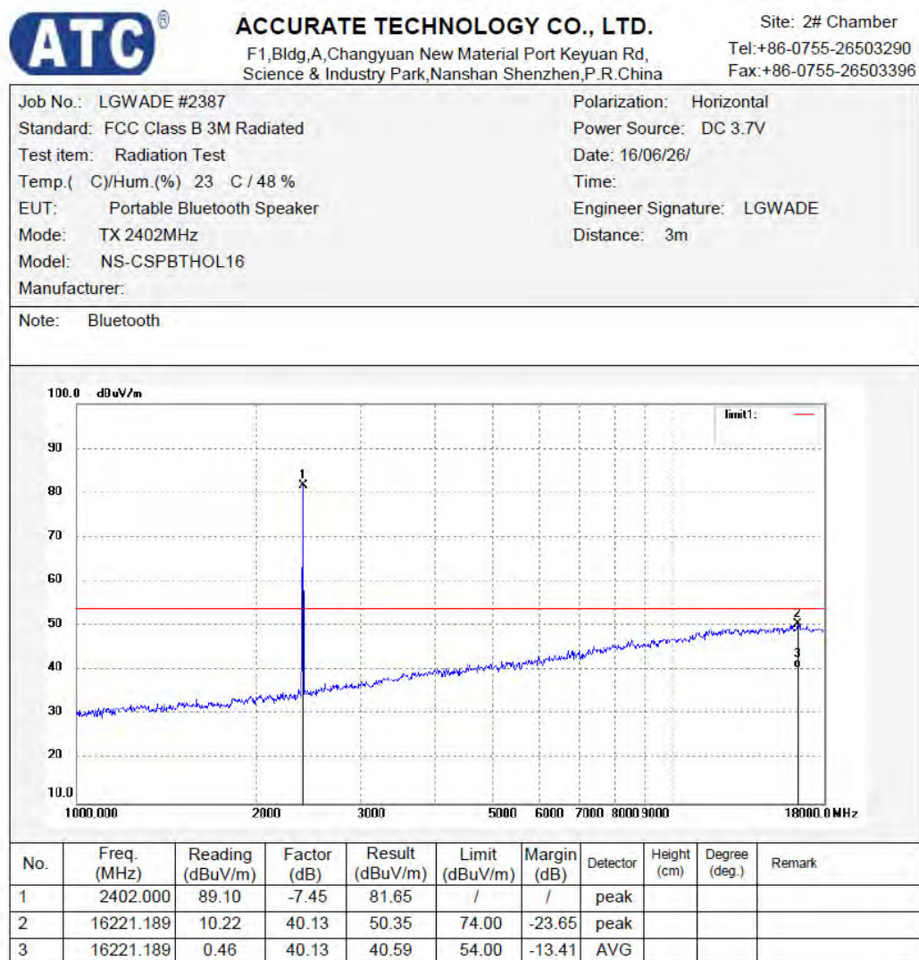
Figure 5: Test figure of spurious emissions, mode A.1, Horizontal polarity (1GHz –18GHz)
