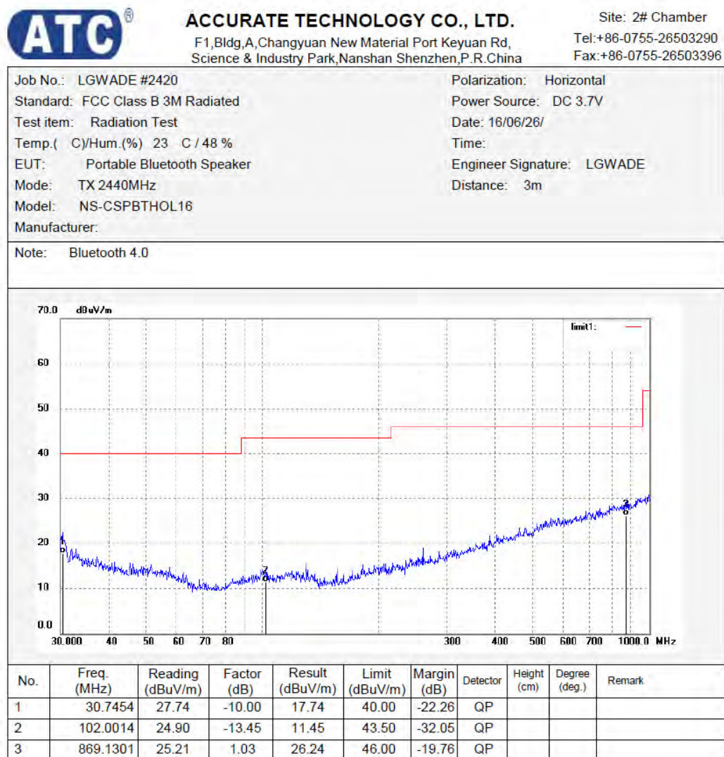
Figure 35: Test figure of spurious emissions, mode B.2, Horizontal polarity (30MHz – 1GHz)
